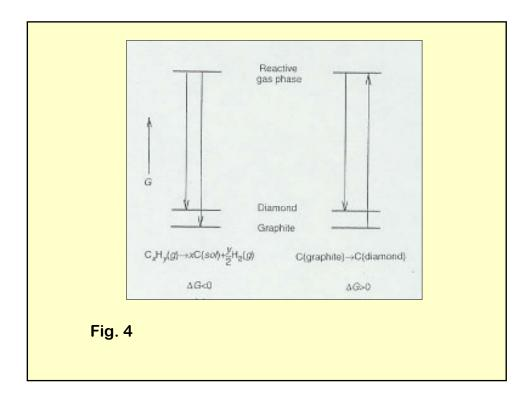
The simultaneous CVD of diamond and gasification of graphite is recognized as the vapor-phase transport of carbon from graphite to diamond. Summing Eqs. (5) and (6) to obtain an overall process gives
