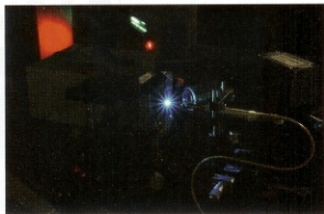
A blue photonic-quantum-ring laser showcases 3-D whispering-cave-mode emission with ultralow threshold current less than that of VCSELs or LEDs. (Courtesy of Odae Kwon, POSTECH)
