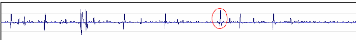
Channel 1 - Channel 2: reference applied to remove the artifact
