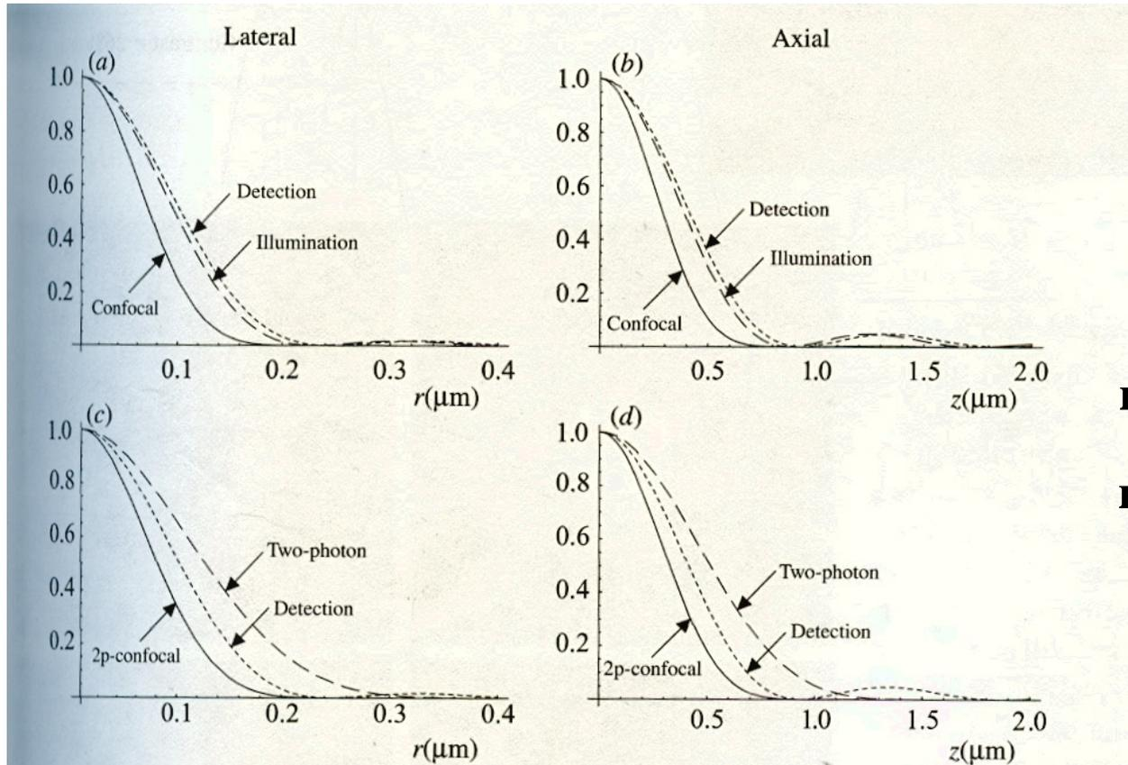
$$r_{xy,\text{confocal}} \approx 0.4 \lambda / \text{NA}$$
