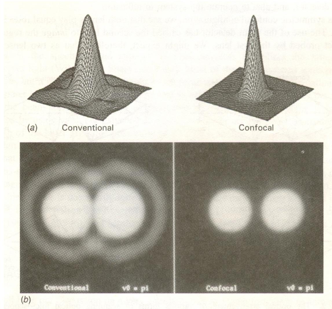
Comparison of (a) Point spread function, (b) two-point objects image
