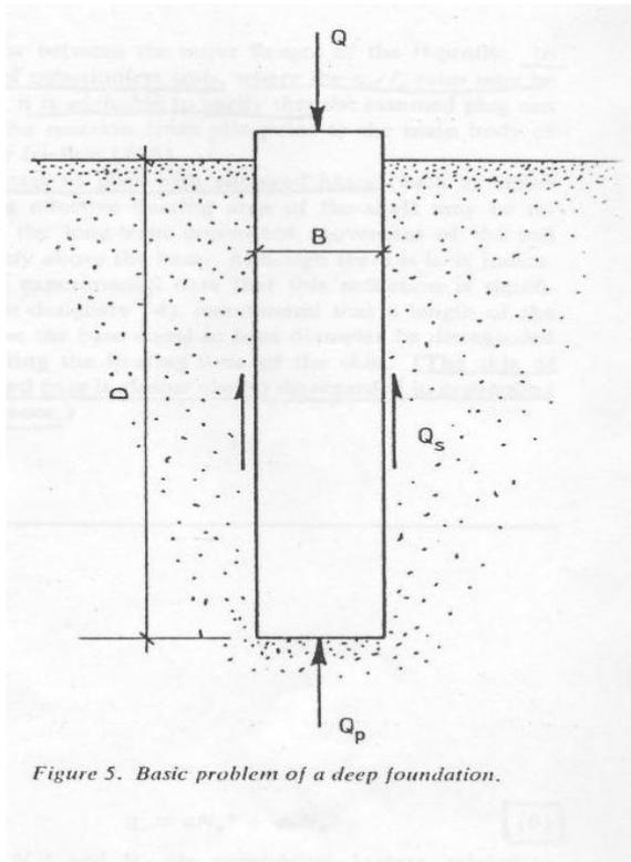
: A cylinder shaft of diameter  $B$  is placed to depth  $D$  inside a soil mass of known physical properties ( $c$ ,  $\phi$ ,  $\gamma$ ). a static, vertical and central load  $Q$  is applied at the top and increased until a shear failure in the soil is produced. the problem is to determine the ultimate load  $Q_0$  that this foundation can support.
