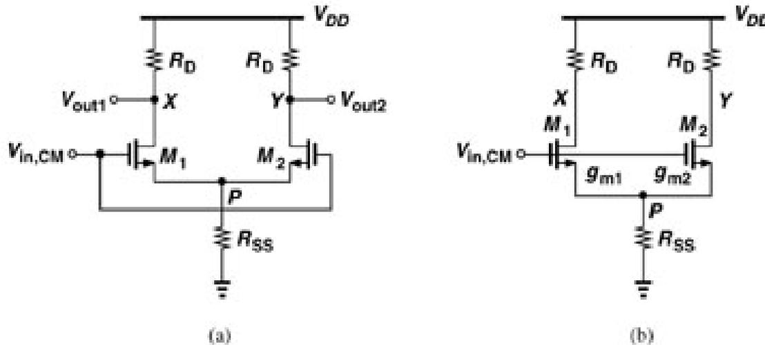
$$A_{V,CM-DM} = \frac{V_X - V_Y}{V_{in,CM}} = - \frac{g_{m1} - g_{m2}}{(g_{m1} + g_{m2})R_{SS} + 1} R_D$$
