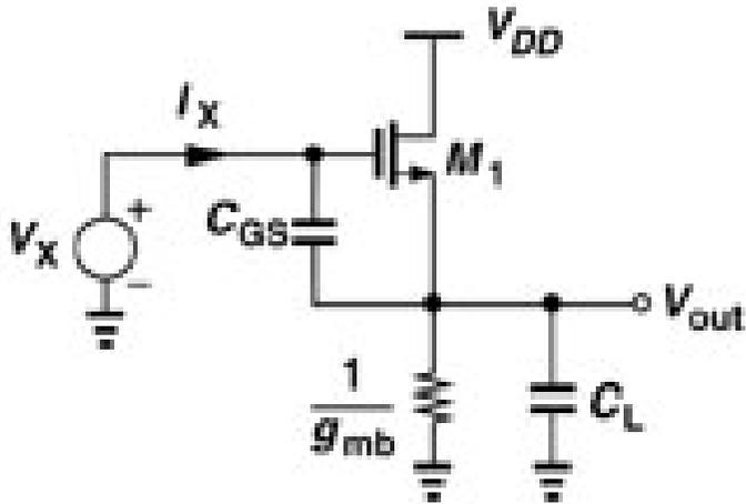
Laying  $C_{GD}$  aside, as it appears in parallel to the remaining part of  $Z_{in}$ :
