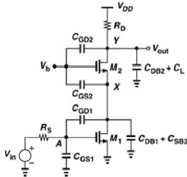
$$f_{p,A} = \frac{1}{2\pi R_S \left[ C_{GS1} + \left( 1 + \frac{g_{m1}}{g_{m2} + g_{mb2}} \right) C_{GD1} \right]}$$
