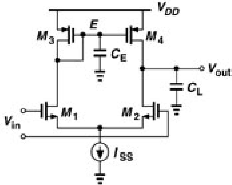
$C_E$  arises from  $C_{GS3}$ ,  $C_{GS4}$ ,  $C_{DB3}$ ,  $C_{DB1}$  and Miller effect of  $C_{GD1}$  and  $C_{GD4}$ . Pole is at  $s = -g_{m3}/C_E$
