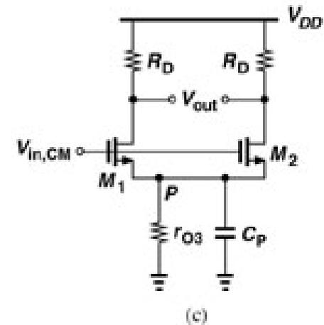
Do separate Differential-Mode and Common-Mode high-frequency response analysis
