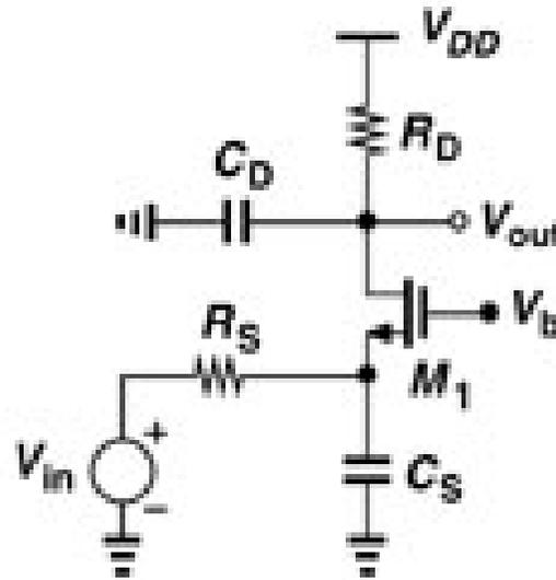
Can we use Miller's theorem for the bridging  $r_o$  resistor? Well, no.
