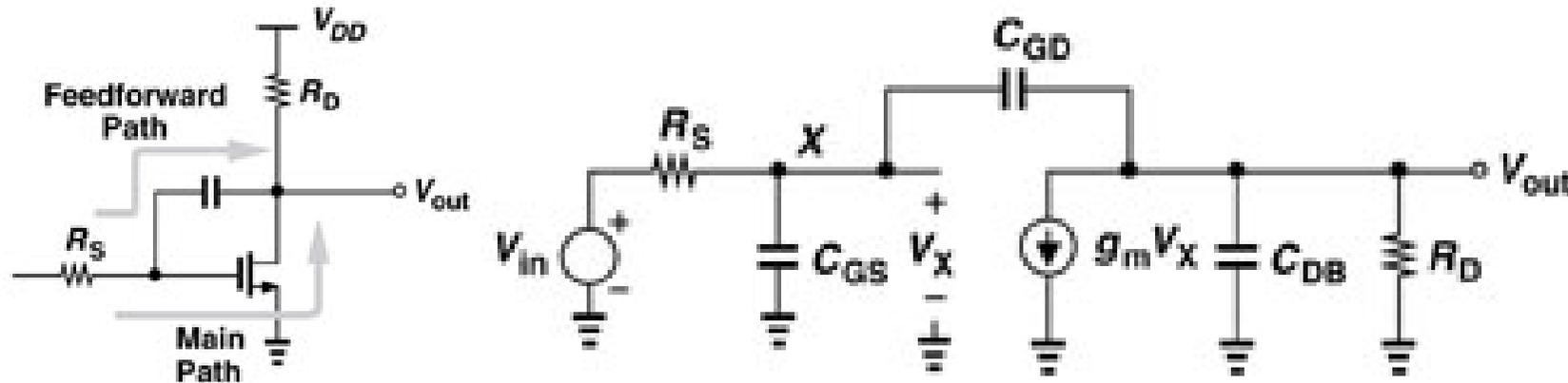
$$\frac{V_{out}(s)}{V_{in}(s)} = \frac{(sC_{GD} - g_m)R_D}{s^2 R_S R_D (C_{GS} C_{GD} + C_{GS} C_{SB} + C_{GD} C_{DB}) + s [R_S (1 + g_m R_D) C_{GD} + R_S C_{GS} + R_D (C_{GD} + C_{DB})] + 1}$$
