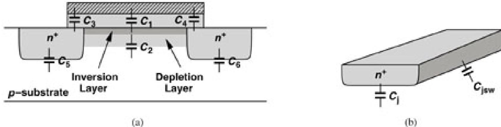
In MOSFET models  $C_j$  and  $C_{jsw}$  are usually given as capacitance-per-unit-area, and capacitance-per-unit-length, respectively.
