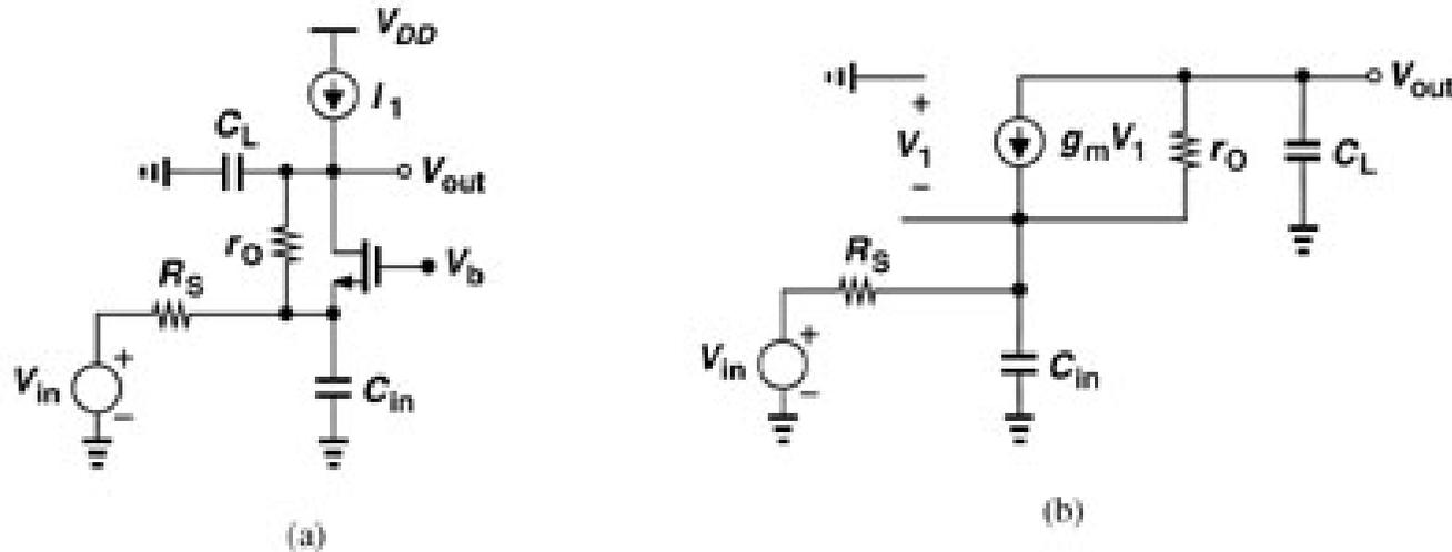
$$Z_{in} = [1/sC_L / ((g_m + g_{mb})r_o)] + [1/(g_m + g_{mb})].$$
