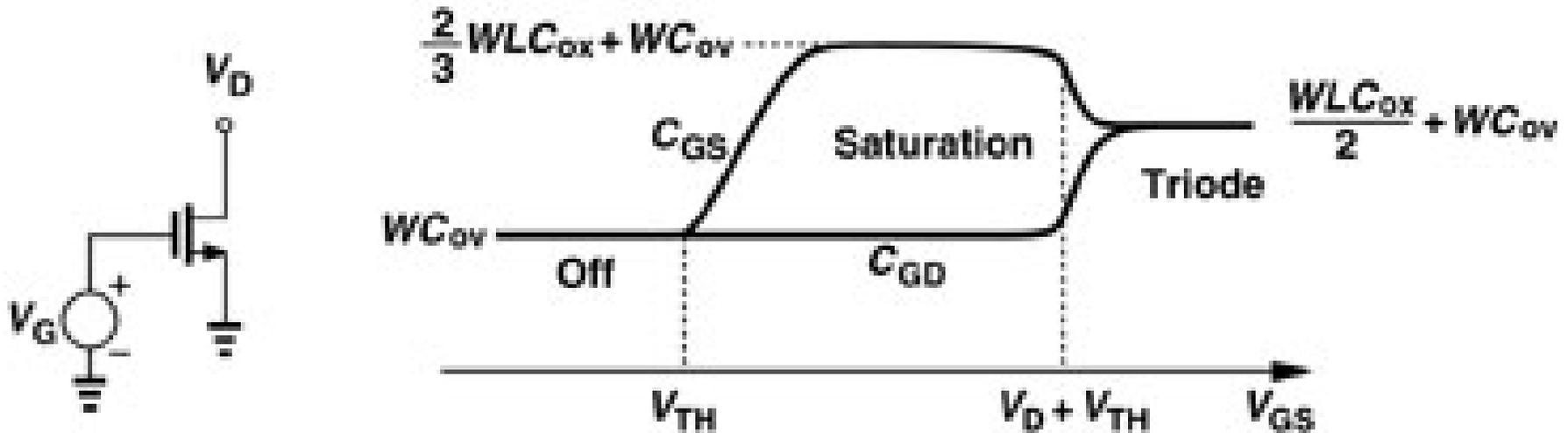
$$C_{GD} = C_{GS} = C_{ov}W$$
