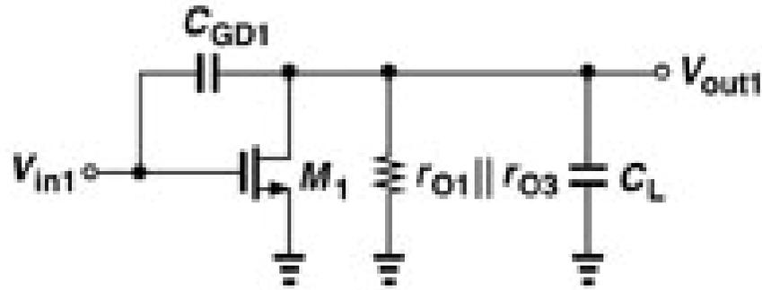
$$\frac{V_{out}(s)}{V_{in}(s)} = \frac{(sC_{GD} - g_m)R_D}{s^2 R_S R_D (C_{GS} C_{GD} + C_{GS} C_{SB} + C_{GD} C_{DB}) + s [R_S (1 + g_m R_D) C_{GD} + R_S C_{GS} + R_D (C_{GD} + C_{DB})] + 1}$$
