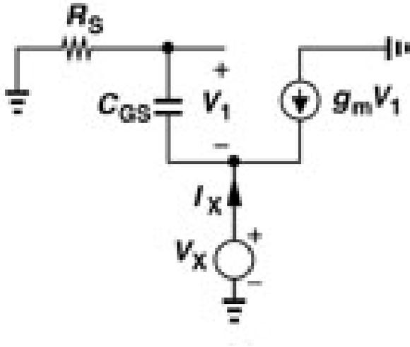
Body effect and  $C_{SB}$  contribute an impedance which is a parallel portion of  $Z_{out}$  – we'll keep it in mind. We also neglect  $C_{GD}$ .
