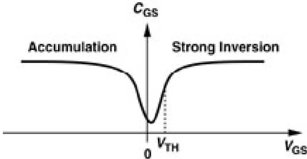
In “Weak Inversion”  $C_{GS}$  is a series combination of  $C_{OX}$ -capacitance and  $C_{dep}$ -capacitance  $\rightarrow$  Low capacitance peak near  $V_{GS} \approx V_{TH}$
