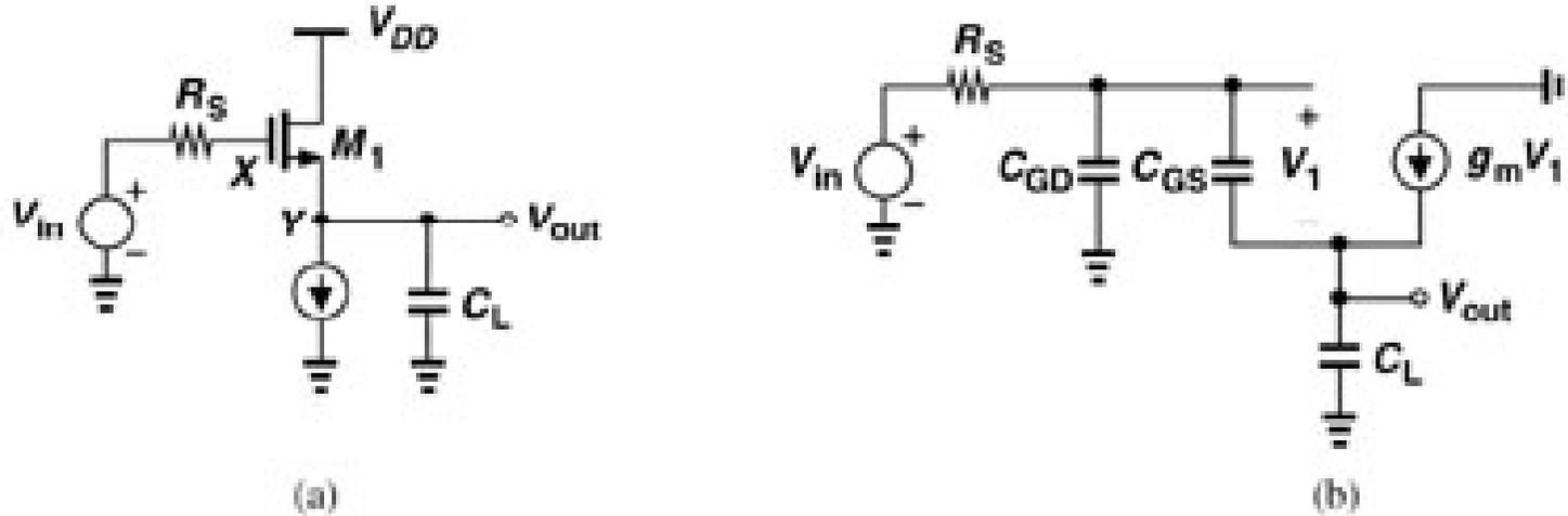
$$\frac{V_{out}(s)}{V_{in}(s)} = \frac{g_m + sC_{GS}}{s^2 R_S (C_{GS} C_L + C_{GS} C_{GD} + C_{GD} C_L) + s(g_m R_S C_{GD} + C_{GD} + C_{GS}) + g_m}$$
