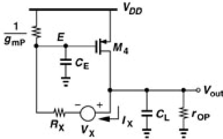
$$\frac{V_{out}}{V_{in}} = \frac{g_{mN} r_{oN} (2g_{mP} + C_E s)}{2r_{oP} r_{oN} C_E C_L s^2 + a s + 2g_{mP} (r_{oN} + r_{oP})}$$
