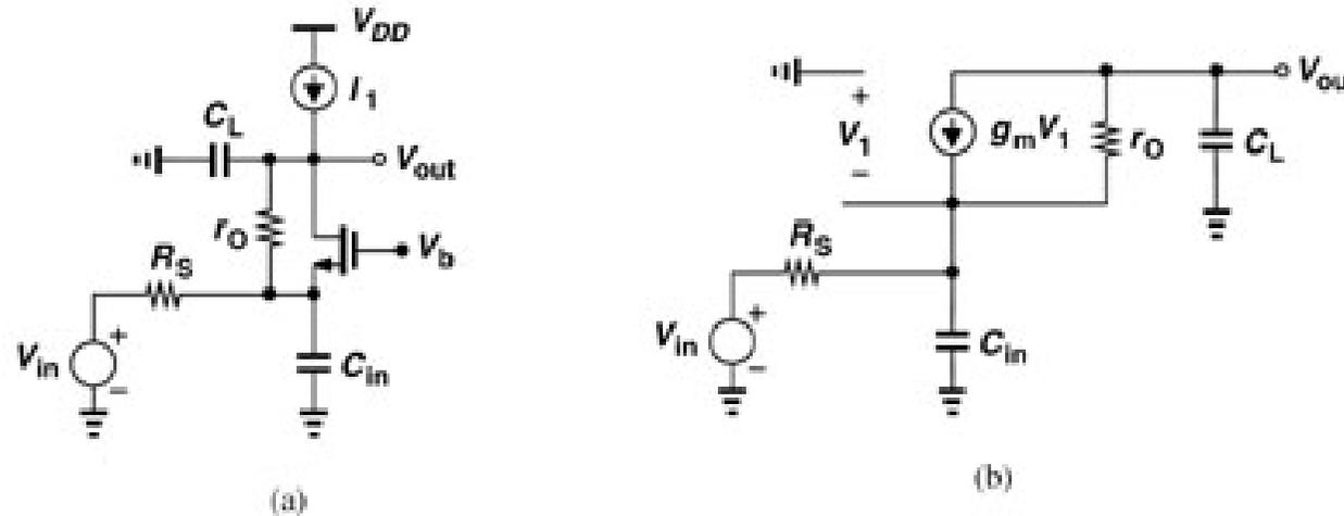
$V_{out}(s)/V_{in}(s) = (1 + g_m r_o) / D(s)$ , where:
