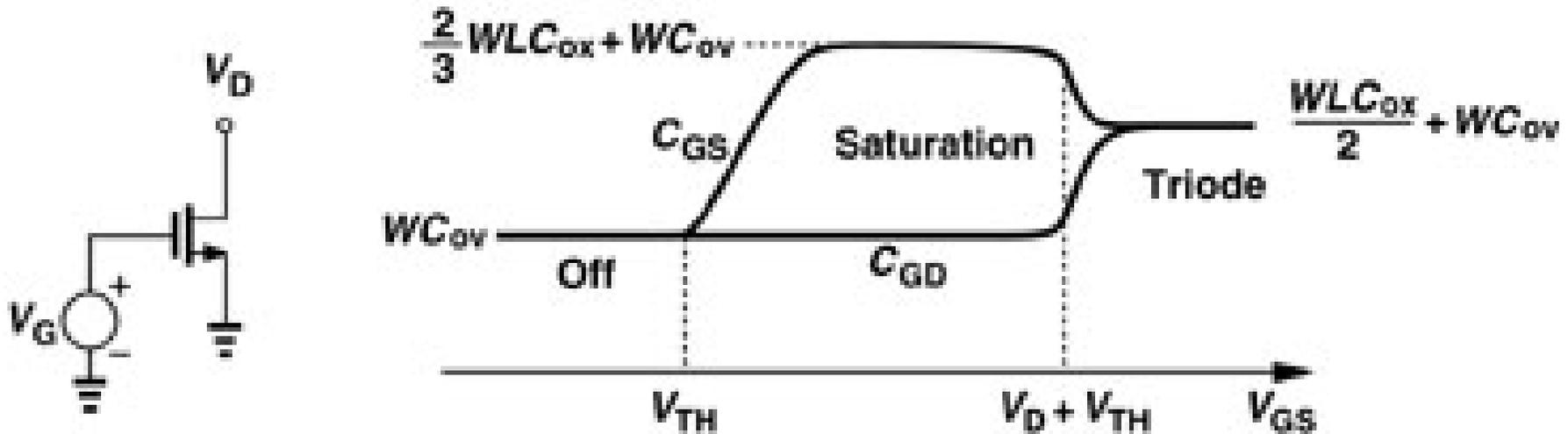
If  $V_{DS}$  is small enough, we can assume  $V_{GS} \approx V_{GD} \rightarrow$  Channel uniform  $\rightarrow$  Gate-Channel capacitance  $WLC_{OX}$  is distributed uniformly
