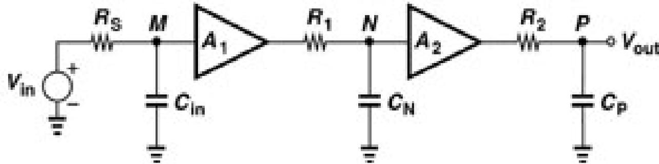
$$\frac{V_{out}(s)}{V_{in}(s)} = \frac{A_1 A_2}{(1 + sR_S C_{in})(1 + sR_1 C_N)(1 + sR_2 C_P)}$$
