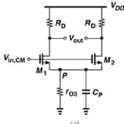
$C_P$  depends on  $C_{GD3}$ ,  $C_{DB3}$ ,  $C_{SB1}$  and  $C_{SB2}$
