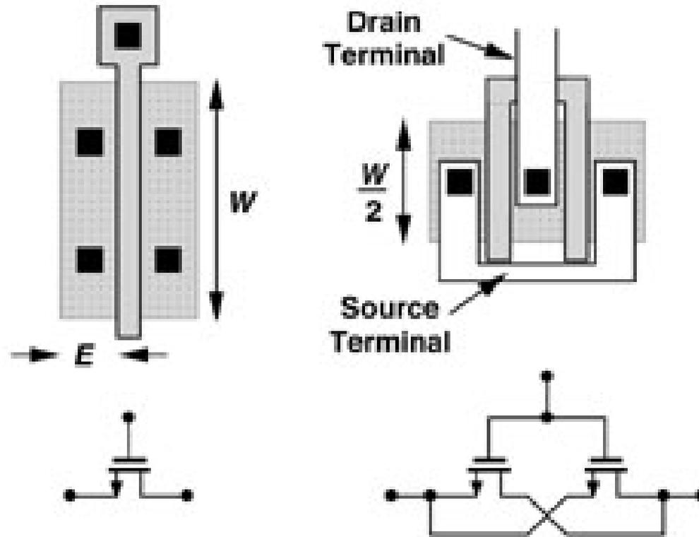
Two parallel transistors with one common Drain
