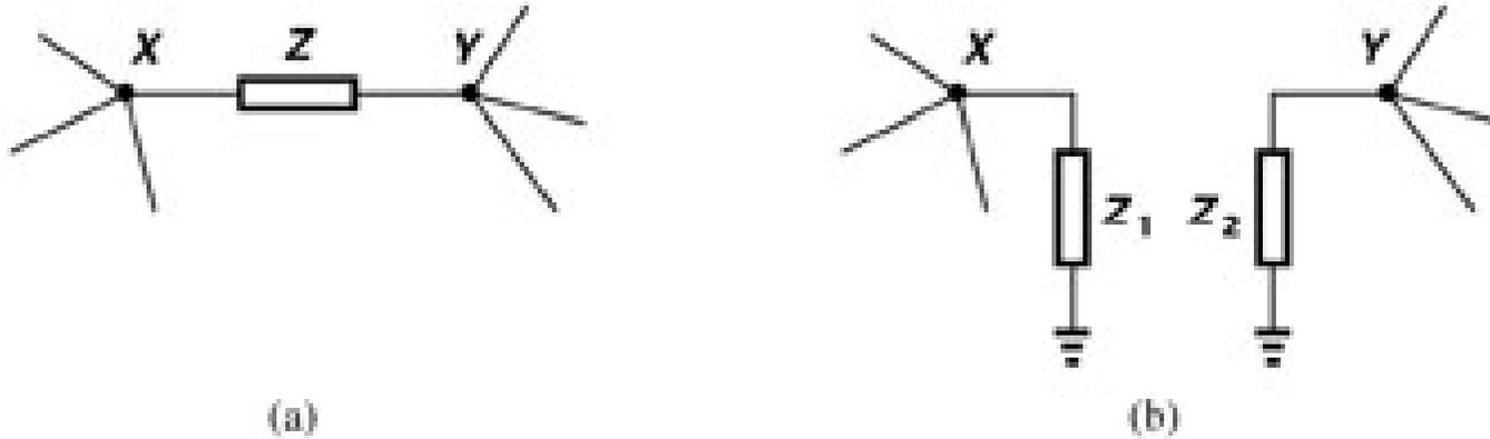
Replacement of a bridging component (typically a capacitor) with equivalent input and output impedances, for the sake of facilitating high-frequency response analysis.
