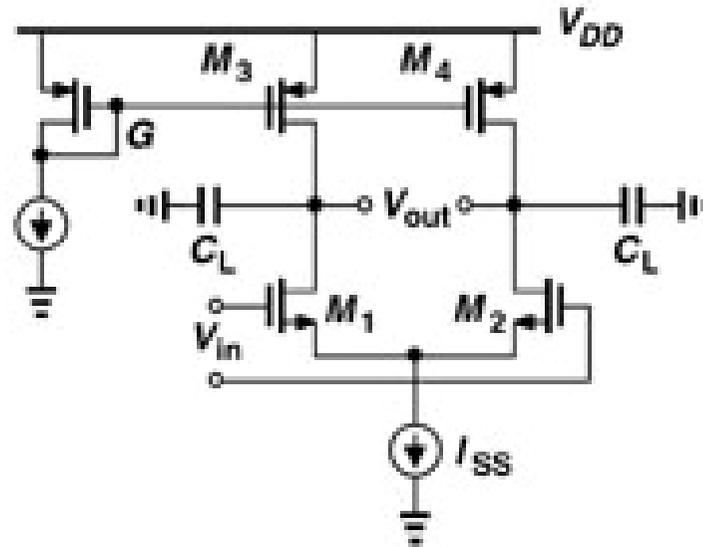
Here  $C_L$  include  $C_{GD}$  and  $C_{DB}$  of PMOS loads
