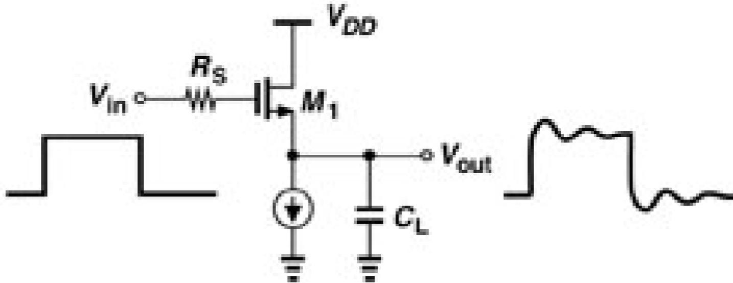
Output ringing due to tuned circuit formed with  $C_L$  and inductive component of output impedance. It happens especially if load capacitance is large.
