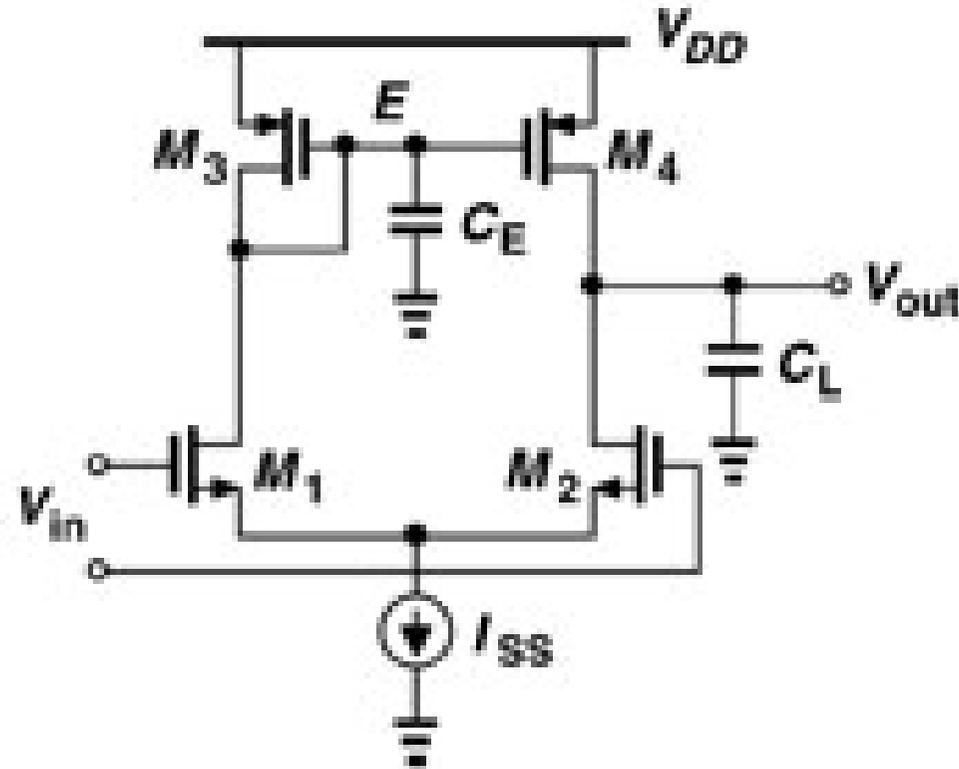
Solution approach: Replace  $V_{in}$ ,  $M_1$  and  $M_2$  by a Thevenin equivalent
