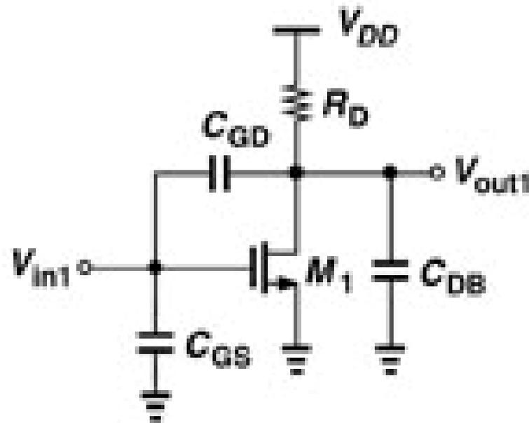
Differential-Mode HF response identical to that of a CS amplifier.
