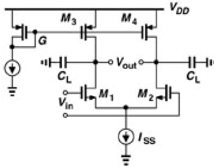
Result identical to that of a differential amplifier with  $R_D$  load.
