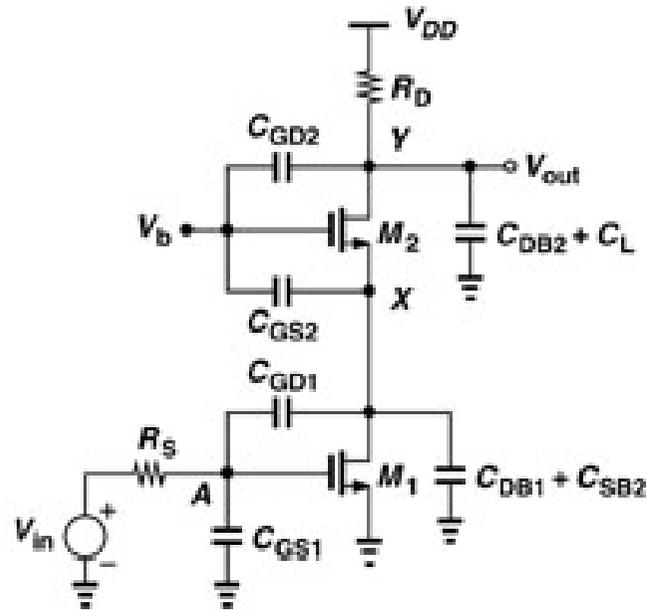
$$f_{p,Y} = \frac{1}{2\pi R_D (C_{DB2} + C_L + C_{GD2})}$$
