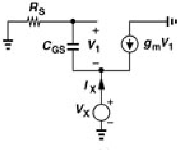
If  $|Z_{out}(\omega)|$  is increasing with  $\omega$ , then it must have an **INDUCTIVE** component!
