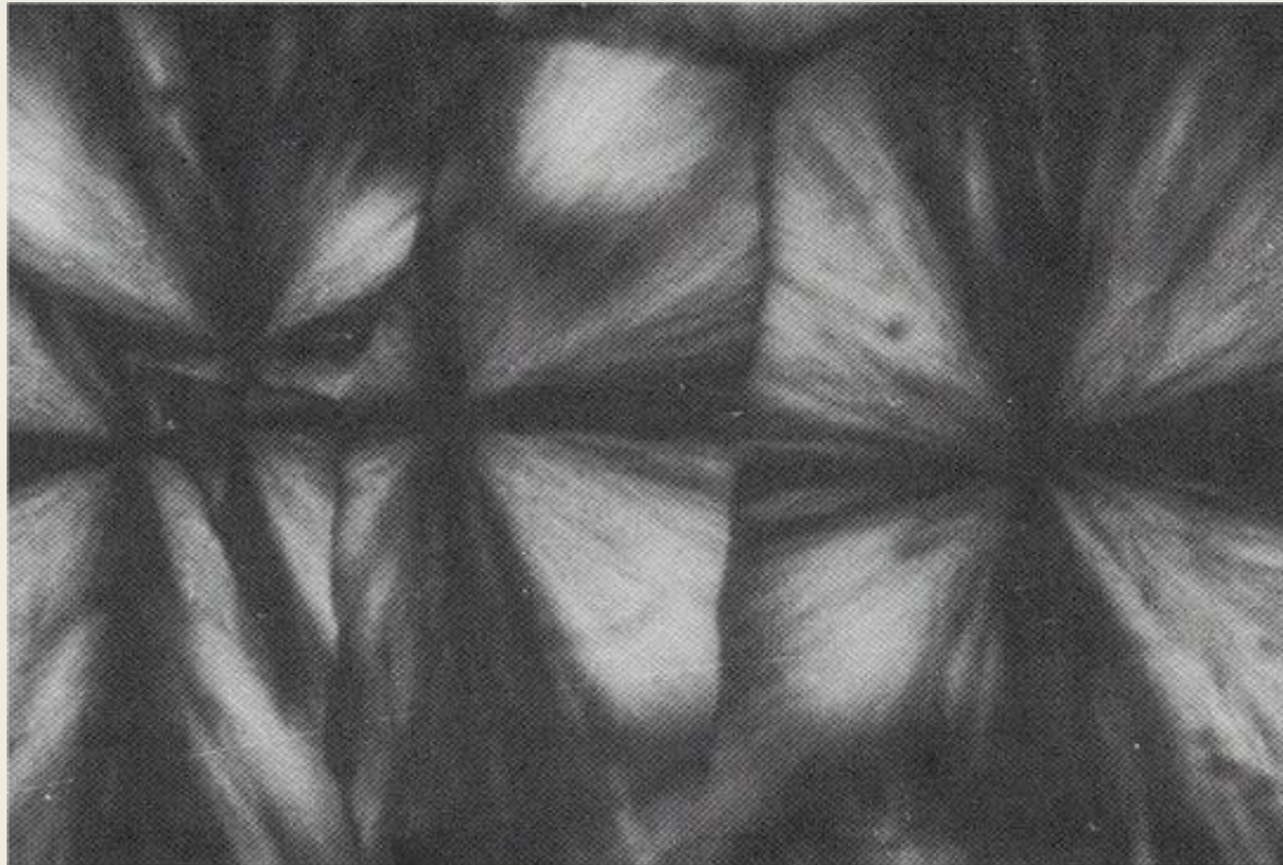
Fig. 6.4 Spherulites of low-density polyethylene, observed through crossed polarizers. Note characteristic Maltese cross pattern.
