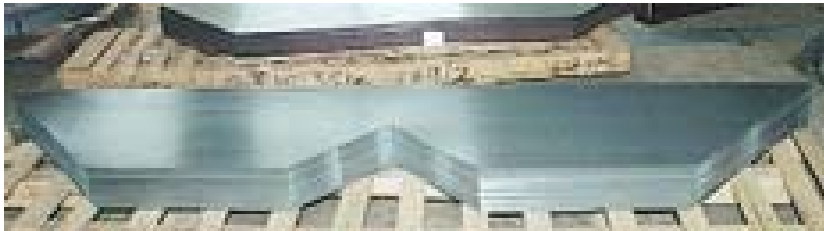
Stacked transformer core
