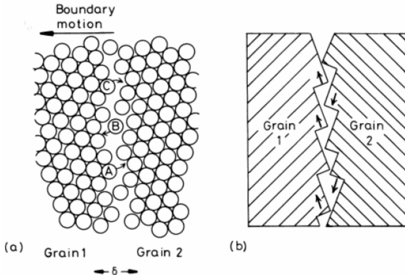
Fig. 3.23 (a) The atomic mechanism of boundary migration. The boundary migrates to the left if the jump rate from grain 1  $\rightarrow$  2 is greater than 2  $\rightarrow$  1. Note that the free volume within the boundary has been exaggerated for clarity. (b) Step-like structure where close-packed planes protrude into the boundary.
