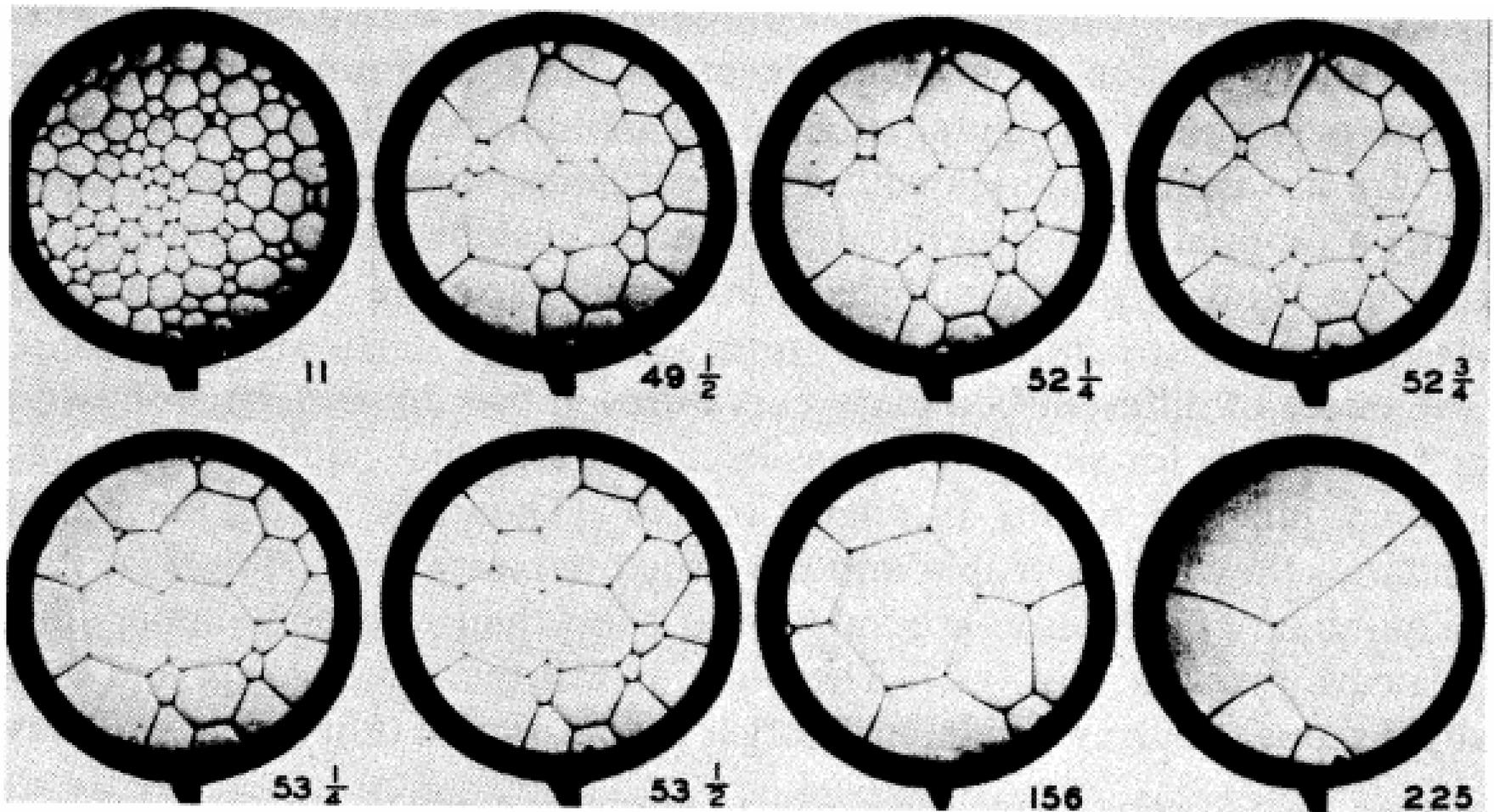
Fig. 3.22 Two-dimensional cells of a soap solution illustrating the process of grain growth. Numbers are time in minutes. (After C.S. Smith, *Metal Interfaces*, American Society for Metals, 1952, p. 81.)
