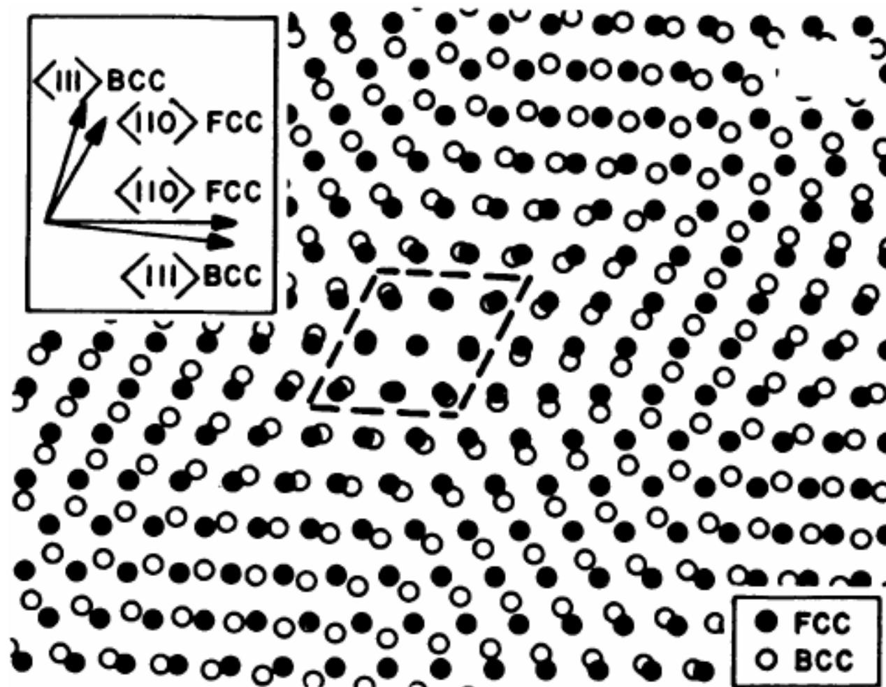
Fig. 3.38 Atomic matching across a  $(111)_{\text{fcc}} / (11)_{\text{bcc}}$  interface bearing the NW orientation relationship for lattice parameters closely corresponding to the case of fcc and bcc iron. (M.G. Hall *et al.*, *Surface Science*, 31 (1972)257).
