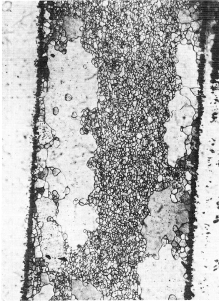
**Figure 5.87** Optical micrograph showing abnormal grain growth in a fine grain steel containing 0.4 wt% carbon. The matrix grains are prevented from growing by a fine dispersion of carbide particles that are not revealed. Magnification  $\times 135$ . (After Gawne and Higgins 1971. Courtesy of the Metals Society.)
