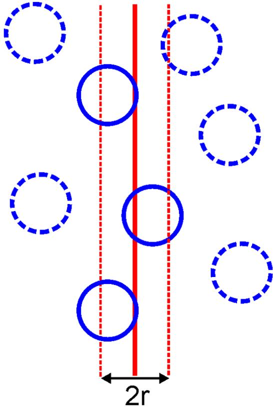
Only particles within one radius (solid circles) can intersect a planar boundary
