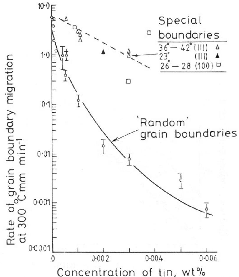
Migration rate of special and random boundaries at 300 °C in zone-refined lead alloyed with tin under equal driving forces
