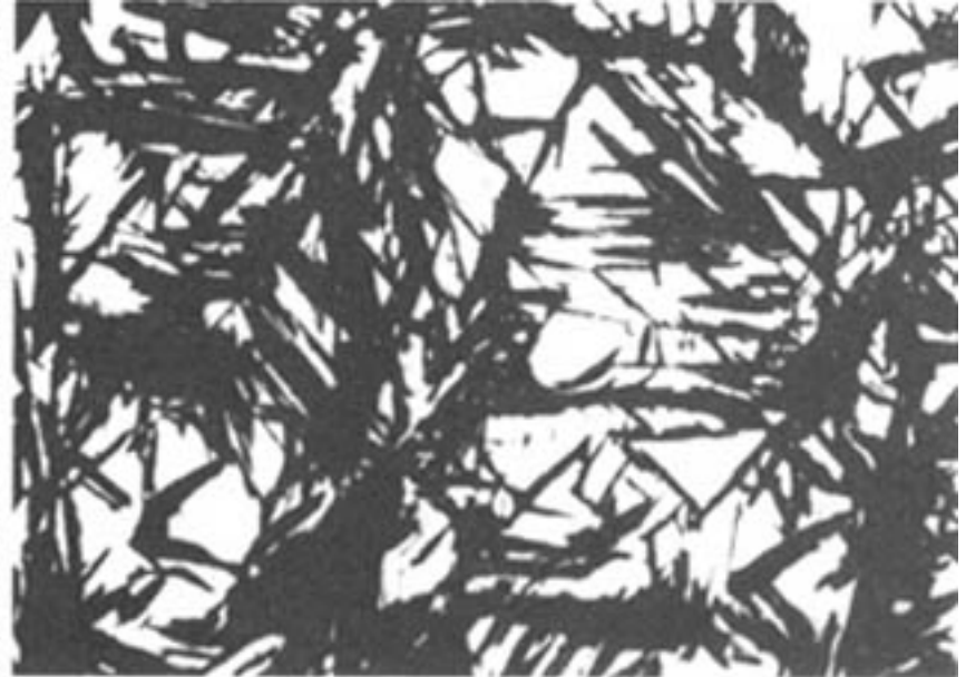
"Needle like" Structure of martensite
