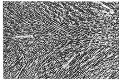
Fig. 4.50 (a) TIG weld of nickel, illustrating low crystal growth speed \times 25 ( by Gudrun Keikkala, University of Lulea, Sweden). (b) Submerged arc weld of steel, illustrating high growth speed \times 24 ( by H. Astrom, University of Lulea, Sweden).
