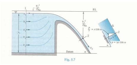
Pressure and velocity on the spillway surface at 2?
