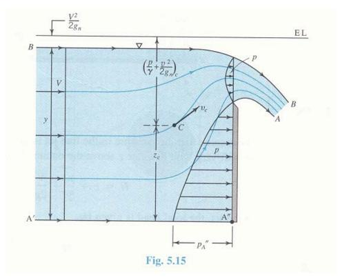
At upstream side, pressure is hydrostatic.
