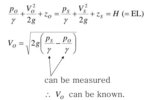
(5) Overflow structure (e.g. spillway of a dam)
