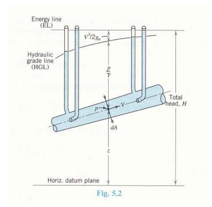
Assumption: The stream tube is infinitesimally thin, so that it can be assumed to be a streamline.
