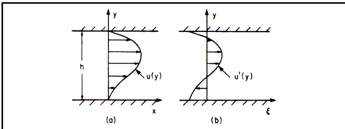
(a) example velocity distribution (b) transformed coordinate system moving at the mean velocity
