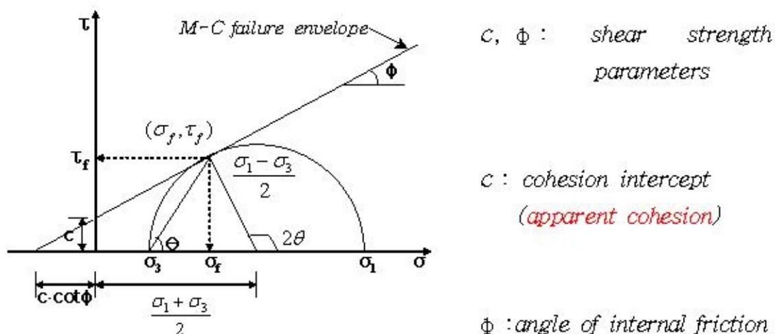
\* How do we get the M-C Failure Envelope ?
