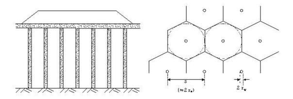
$r_{\it equivalent}$   $(r_e)$  : max, radial drainage path
