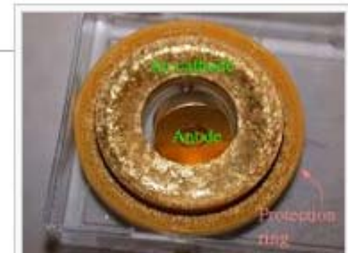
A typical ring-geometry sputter target, here gold showing the cathode made of the material to be deposited, the anode counter-electrode and an outer ring meant to prevent sputtering of the hearth that holds the target.
