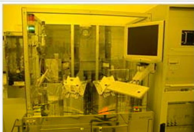
EVG 120 fully automated photoresist coater-developer under inactinic light at LAAS technological facility in Toulouse, France.
