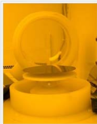
A spin coater (Laurell Technologies model shown) used to apply photoresist to the surface of a silicon wafer.
