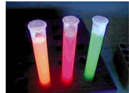
Fig. 3. Luminescence from CdSe @ ZnS QD-glasses formed from TMOS hydrolysis in the presence of octylamine. The gels were 4 days old when photographed under UV light. The QY was estimated to be 0.15 for the red TMOS glasses by comparison to rhodamine (QY = 0.92). Octylamine was used as the surface passivator and sol-gel catalyst. The orange emission was created by mixing red- and green-emitting QDs.
