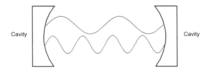
A laser can only lase at those wavelengths (longitudinal modes) for which an integral multiple of half-wavelengths fit into the cavity.
