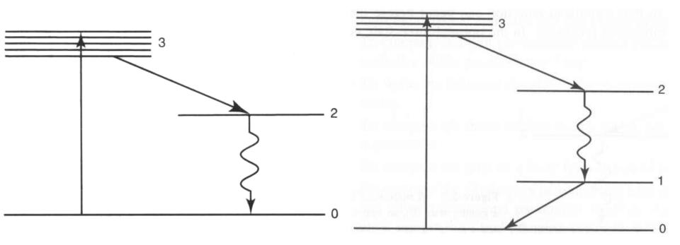
A three-state laser consists of a ground state(0), an upper laser state(2), and a pumping state or states(3).
