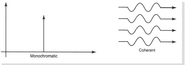
An ideal monochromatic source of light has a group of photons with exactly one frequency. An ideal coherent source of light has a group of photons with the same relative phase.
