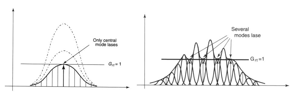
In a homogeneous laser, the entire gain saturates proportionally. As a consequence, only the central longitudinal mode can sustain a round trip gain of 1.
