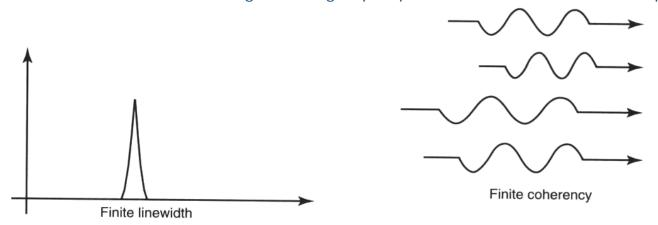
Real laser sources are neither perfectly monochromatic nor perfectly coherent. A real laser will have a finite linewidth and finite coherency.
