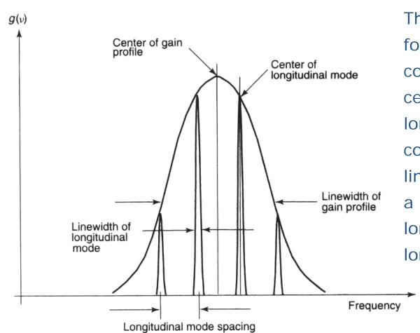
There is a center wavelength for the gain profile and its corresponding frequency, a center wavelength for each longitudinal mode and their corresponding frequencies, a linewidth for the gain profile, a linewidth for each longitudinal mode, and a longitudinal mode separation.
