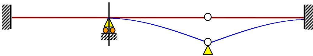
$$M_{BC}^2 = -M_{DC}^2 = \frac{3EI}{l^2} \Delta_C, \quad V_{BC}^2 = -V_{CB}^2 = -\frac{3EI}{l^2} \Delta_C, \quad V_{CD}^2 = -V_{DC}^2 = \frac{3EI}{l^2} \Delta_C$$
