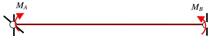
$$\begin{aligned} \frac{L}{3EI}M_A + \frac{L}{6EI}M_B &= -\theta_A \rightarrow M_A = -\frac{4EI}{L}\theta_A, \quad M_B = \frac{2EI}{L}\theta_A \\ \frac{L}{6EI}M_A + \frac{L}{3EI}M_B &= 0 \end{aligned}$$
