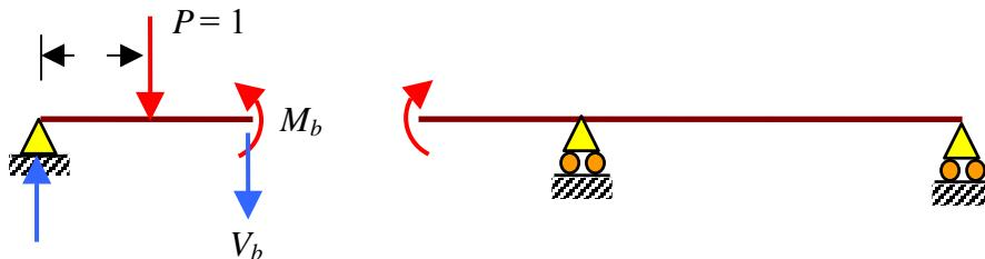
$$V_b \times \frac{L}{2} + 1 \times x - M_b = 0 \rightarrow V_b = \frac{2M_b}{L} - \frac{2x}{L} = \frac{1}{4L^3}(x^3 + 3L^2x) - \frac{2x}{L} = \frac{1}{4L^3}(x^3 - 5L^2x)$$
