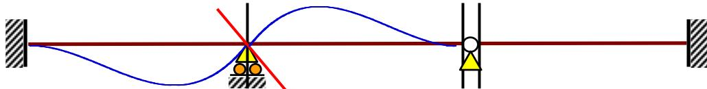
$$M_{AB}^1 = \frac{2EI}{l} \theta_B, \quad M_{BA}^1 = M_{BC}^1 = \frac{4EI}{l} \theta_B, \quad M_{CB}^1 = \frac{2EI}{l} \theta_B, \quad V_{CB}^1 = \frac{6EI}{l^2} \theta_B$$
