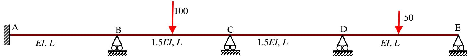
$$D_{BA} = 4 \frac{EI}{L} \left( 4 \frac{EI}{L} + 4 \frac{1.5EI}{L} \right) = 0.4, \quad D_{BC} = 4 \frac{1.5EI}{L} \left( 4 \frac{EI}{L} + 4 \frac{1.5EI}{L} \right) = 0.6, \quad D_{CB} = 4 \frac{1.5EI}{L} \left( 4 \frac{1.5EI}{L} + 4 \frac{1.5EI}{L} \right) = 0.5,$$
