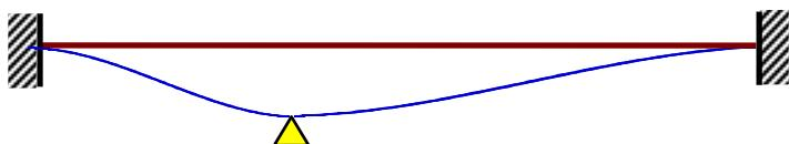
$$M_{AB}^2 = \frac{6EI}{a^2} \Delta_B, \quad M_{BA}^2 = \frac{6EI}{a^2} \Delta_B, \quad M_{BC}^2 = -\frac{6EI}{b^2} \Delta_B, \quad M_{CB}^2 = -\frac{6EI}{b^2} \Delta_B$$
