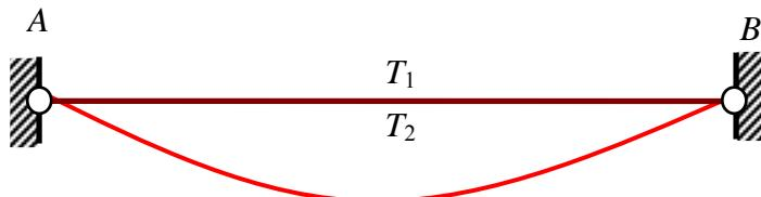
$$\theta_A = \frac{\alpha(T_2 - T_1)}{2h} L, \quad \theta_B = -\frac{\alpha(T_2 - T_1)}{2h} L$$
