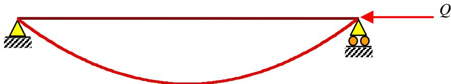
– with a parabola:  $w = ax(x-l) \rightarrow g'_1 = 2x-l, g''_1 = 2$
