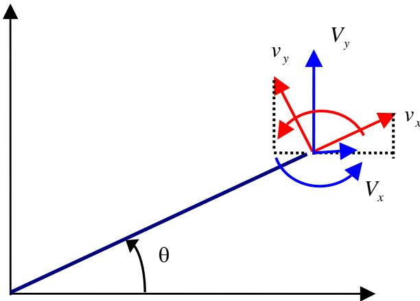
$$\begin{aligned} V_x &= \cos \theta v_x - \sin \theta v_y \\ V_y &= \sin \theta v_x + \cos \theta v_y \\ M &= m \end{aligned} \rightarrow \begin{pmatrix} V_x \\ V_y \\ M \end{pmatrix} = \begin{bmatrix} \cos \theta & -\sin \theta & 0 \\ \sin \theta & \cos \theta & 0 \\ 0 & 0 & 1 \end{bmatrix} \begin{pmatrix} v_x \\ v_y \\ m \end{pmatrix}$$
