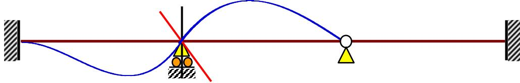
$$M_{AB}^1 = \frac{2EI}{l} \theta_B, \quad M_{BA}^1 = \frac{4EI}{l} \theta_B, \quad M_{BC}^1 = \frac{3EI}{l} \theta_B, \quad -V_{BC}^1 = V_{CB}^1 = \frac{3EI}{l^2} \theta_B$$
