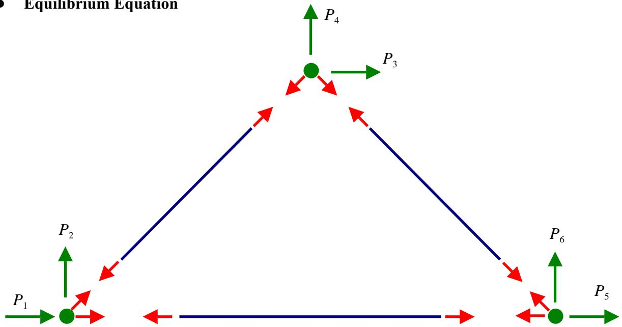
$$\begin{aligned} P_1 &= (F_x^1)^1 + (F_x^2)^3 \\ P_2 &= (F_y^1)^1 + (F_y^2)^3 \\ P_3 &= (F_x^2)^1 + (F_x^1)^2 \\ P_4 &= (F_y^2)^1 + (F_y^1)^2 \\ P_5 &= (F_x^2)^2 + (F_x^1)^3 \\ P_6 &= (F_y^2)^2 + (F_y^1)^3 \end{aligned}$$
