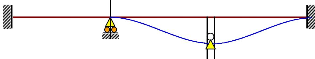
$$M_{BC}^4 = M_{CB}^4 = \frac{6EI}{l^2} \Delta_C, \quad M_{CD}^4 = M_{DC}^4 = -\frac{6EI}{l^2} \Delta_C, \quad V_{CD}^4 = V_{CB}^4 = \frac{12EI}{l^2} \Delta_C$$
