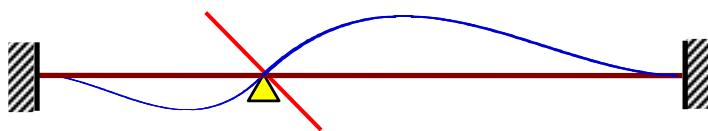
$$M_{AB}^1 = \frac{2EI}{a} \theta_B, \quad M_{BA}^1 = \frac{4EI}{a} \theta_B, \quad M_{BC}^1 = \frac{4EI}{b} \theta_B, \quad M_{CB}^1 = \frac{2EI}{b} \theta_B$$
