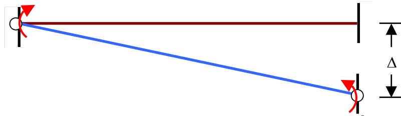
$$\frac{L}{3EI} M_A + \frac{L}{6EI} M_B = -\frac{\Delta}{L} \rightarrow M_A = -\frac{6EI}{L} \frac{\Delta}{L}, \quad M_B = \frac{6EI}{L} \frac{\Delta}{L}$$
