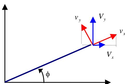
$$\left. \begin{aligned} V_x &= \cos \phi v_x - \sin \phi v_y \\ V_y &= \sin \phi v_x + \cos \phi v_y \end{aligned} \right\} \rightarrow \begin{pmatrix} V_x \\ V_y \end{pmatrix} = \begin{bmatrix} \cos \phi & -\sin \phi \\ \sin \phi & \cos \phi \end{bmatrix} \begin{pmatrix} v_x \\ v_y \end{pmatrix}$$
