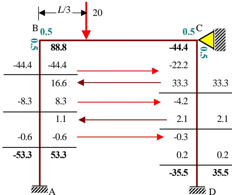
$$M_{AB} = -53.3/2 = -26.7, M_{DC} = -35.5/2 = 17.8, V_{AB} = 2.67, V_{DC} = -1.78, V^P = 0.89$$
