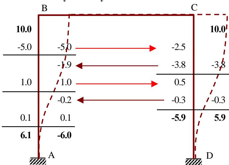
$$M_{AB} = 10 - 3.9/2.0 = 8.1, M_{DC} = 10 - 4.1/2.0 = 7.9, V_{AB} = -0.47, V_{DC} = -0.46, V^{\bar{\Delta}} = -0.93$$
