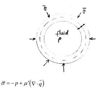
If fluid is compressed, expanded or made to oscillate at a finite rate, work done in a thermodynamically reversible process per unit volume is
