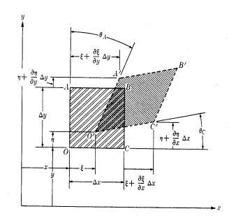
[Re] displacement vs. deformation
