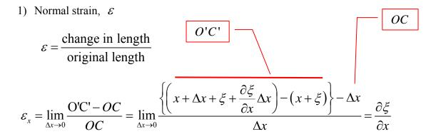
$$\varepsilon_{y} = \lim_{\Delta y \to 0} \frac{O'A' - OA}{OA} = \lim_{\Delta y \to 0} \frac{\left\{ \left( y + \Delta y + \eta + \frac{\partial \eta}{\partial y} \Delta y \right) - \left( y + \eta \right) \right\} - \Delta y}{\Delta y} = \frac{\partial \eta}{\partial y}$$
