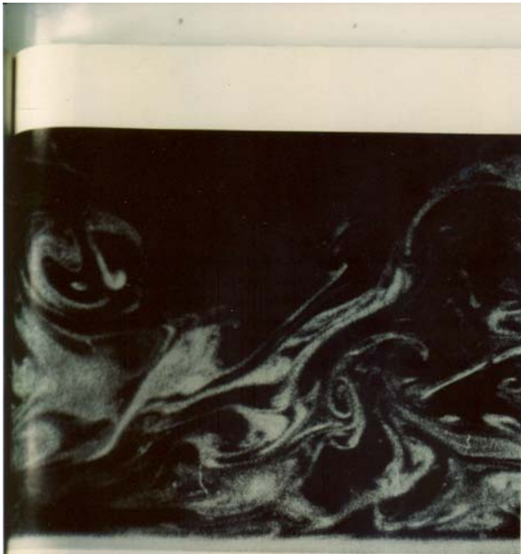
162. "Typical eddy" in a turbulent boundary layer. Oil fog is illuminated by a sheet of laser light to show the lower two-thirds of a turbulent boundary layer in side view. The vortex-ring structure just below and to the right of center, which resembles a sliced mushroom leaning left, is an example of what Falcó has called a " typical eddy ." It scales on wall variables (figure 161) rather than on the boundary-layer thickness. Photograph by R. E. Falcó
