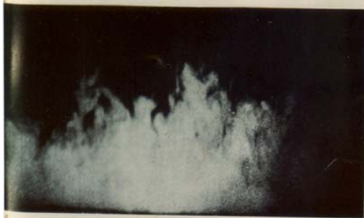
163. Oblique transverse sections of a turbulent boundary layer. The flow is viewed head-on, with smoke illuminated by a sheet of light that is inclined 45^\circ downstream from the wall on the left and 45^\circ upstream on the right.
