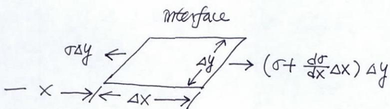
shear force due to surf. tension gradient per unit area
