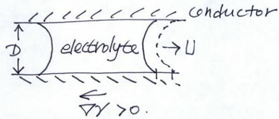
$$\Delta E = [(\gamma_{SL} - \gamma_{SG})_A - (\gamma_{SL} - \gamma_{SG})_R] dx < 0.$$
