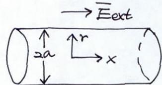
$$\frac{\mu}{r} \frac{\partial}{\partial r} (r \frac{\partial u}{\partial r}) = \frac{\partial p}{\partial x} + Fz(c_+ - c_-) \frac{\partial \phi}{\partial x}$$
