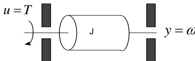
$$J\dot{\omega} + b\omega = T \quad \frac{Y}{U} = \frac{\omega}{T} = \frac{1}{Js + b}$$
