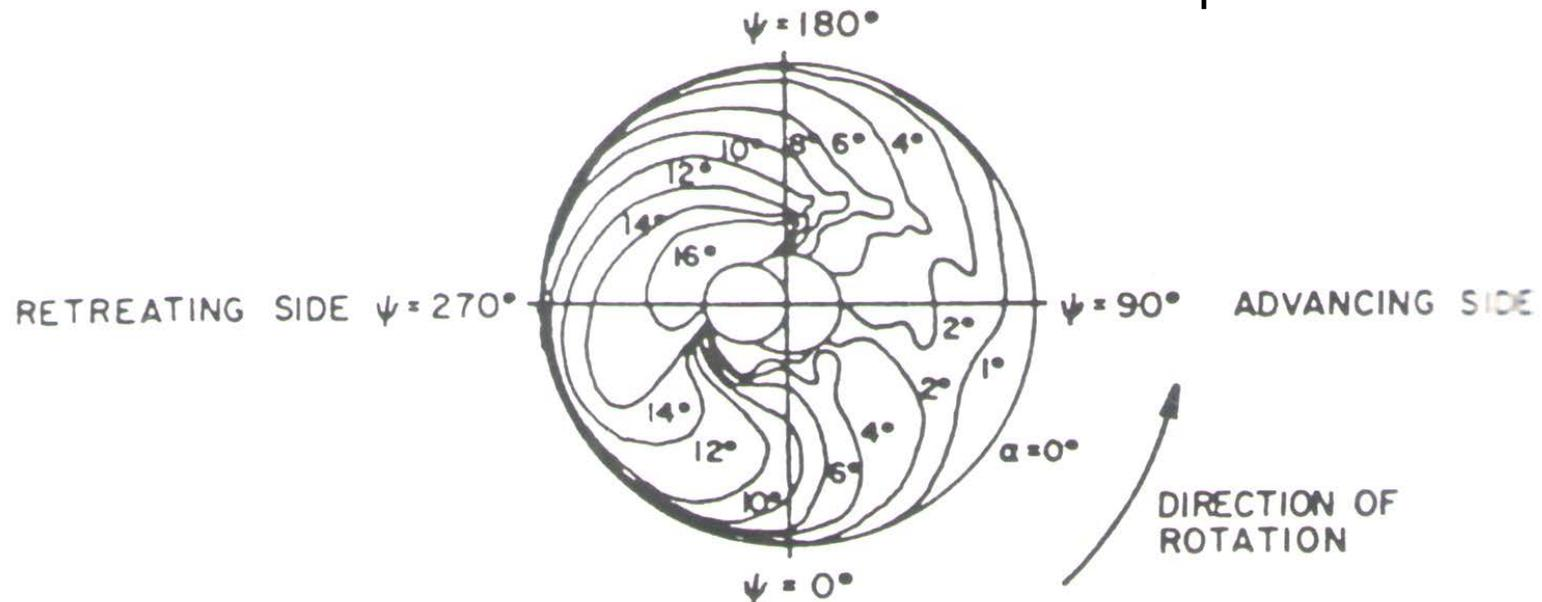
*A.O.A distribution of helicopter rotor at 140 knots ( $\mu = 0.33$ )*
