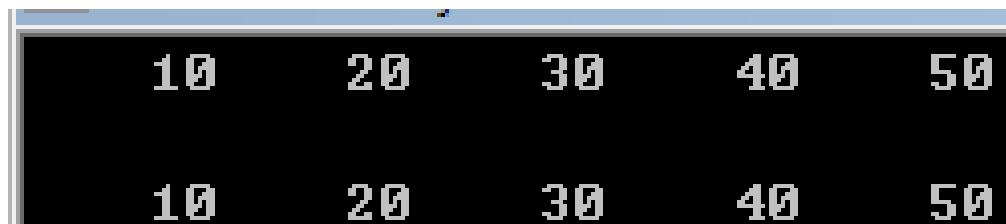
A terminal window showing the execution of a C program. The output consists of two rows of five integers each, separated by spaces. The first row represents the elements of the array ary, and the second row represents the elements of a modified array starting from the third element of ary.
