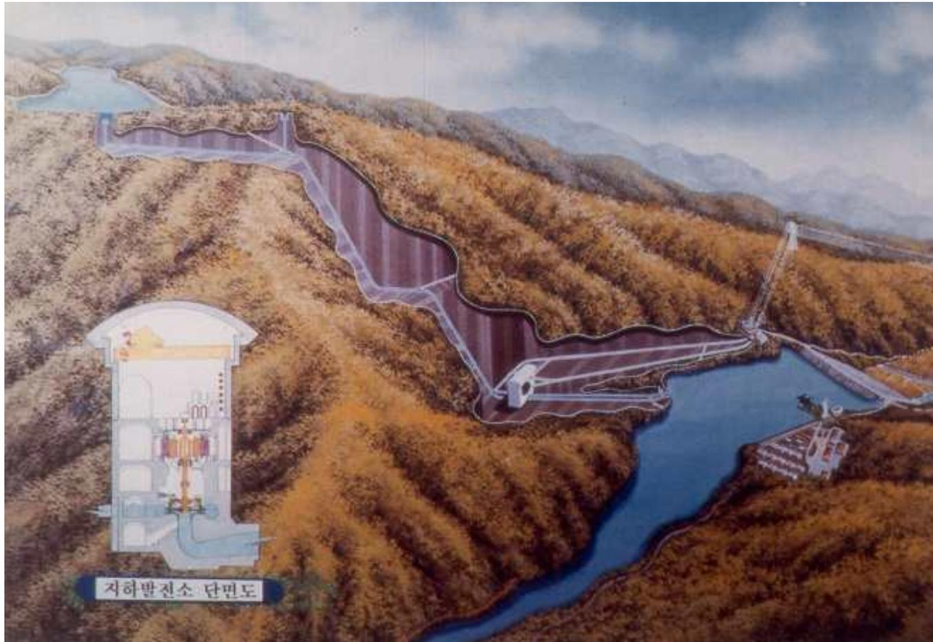
Layout of Muju pumped storage power plant
