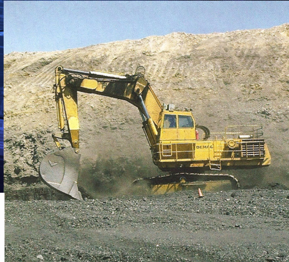
Figure 15.9 Mining coal Large backhoe at the Trapper Mine, Colorado, removing the coal and loading it into large trucks for delivery to a power plant just off the mining site. (Edward A. Keller)
