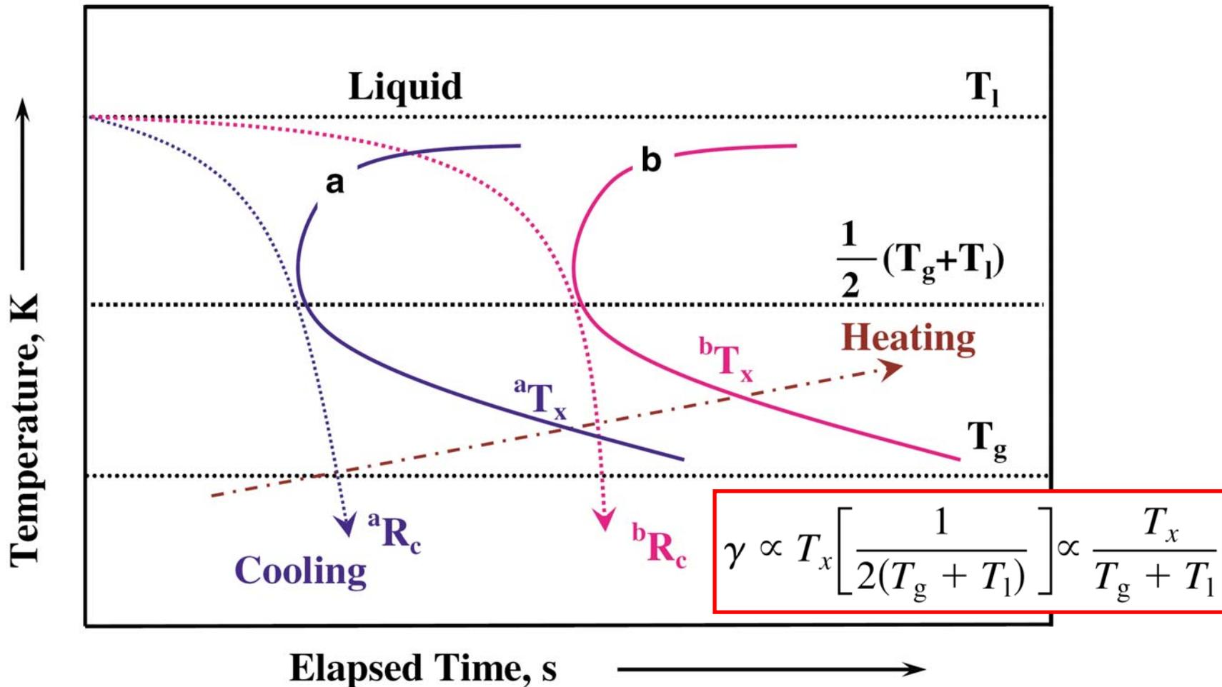
FIG. 2 (color online). Schematic TTT curves showing the effect of  $T_x$  measured upon continuous heating for different liquids with similar  $T_1$  and  $T_g$ ; liquid  $b$  with higher onset crystallization temperature  ${}^bT_x$  ( ${}^aT_x < {}^bT_x$ ) shows a lower critical cooling rate  ${}^bR_c$  ( ${}^bR_c < {}^aR_c$ ).
