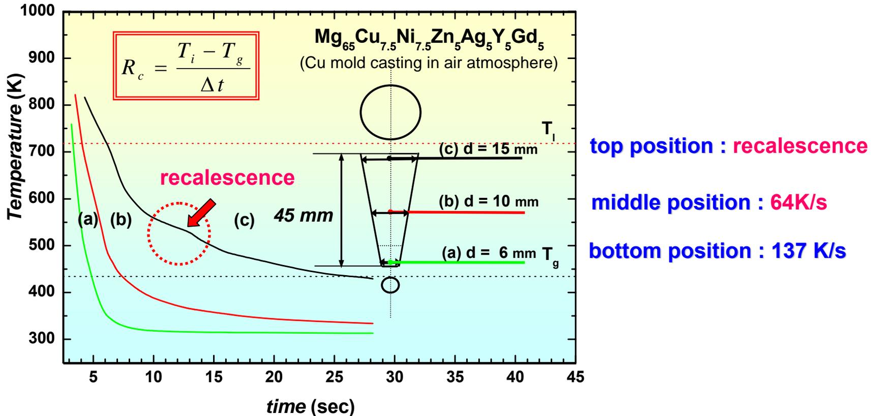
\* Cooling curves measured at the center of the three transverse cross sections
