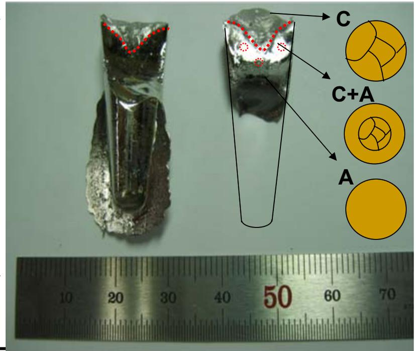
Critical cooling rate is inversely proportional to the diameter of ingot.
