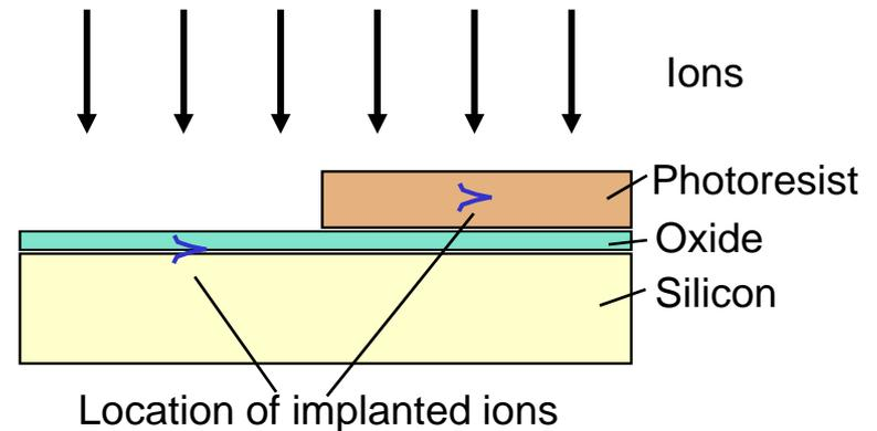
Illustrating the use of a photoresist mask to keep the implant from reaching the silicon in selected regions
