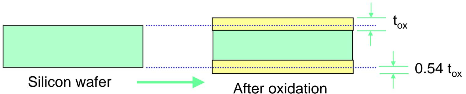
Thermal oxidation consumes some of the wafer thickness. Only 54% of the final oxide thickness appears as a net increase in wafer thickness. The remaining 46% appears as a conversion of silicon to oxide within the original wafer.
