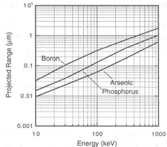
Projected ranges of ions implanted into silicon
