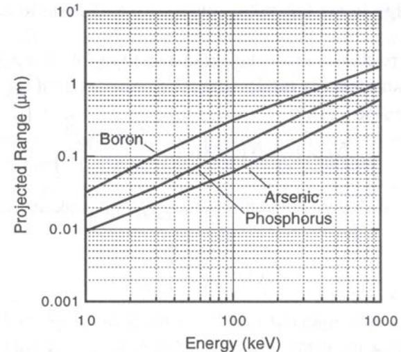
Projected ranges of ions implanted into silicon
