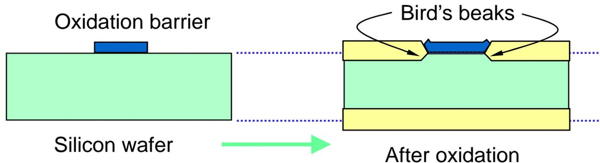
Illustrating selective oxidation of silicon with a silicon nitride thin film serving as an oxidation barrier. In practice, a very thin strain-relief oxide, of order 5 nm thick, is placed beneath the nitride to relieve strains generated during the oxidation process. This oxide is not shown in the diagram.
