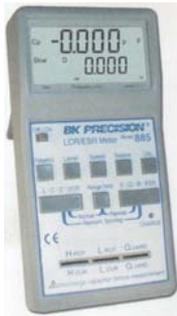
Digital reading capacitance meter.
