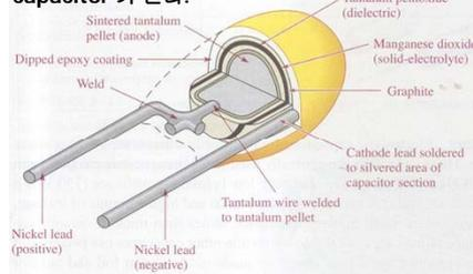
Construction view of a typical "tear drop" shaped tantalum electrolytic capacitor
