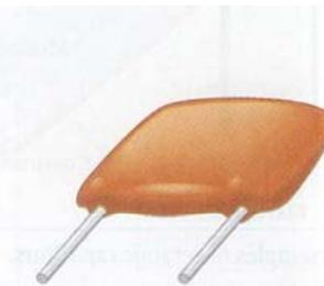
(b) Layers are pressed together and encapsulated.
