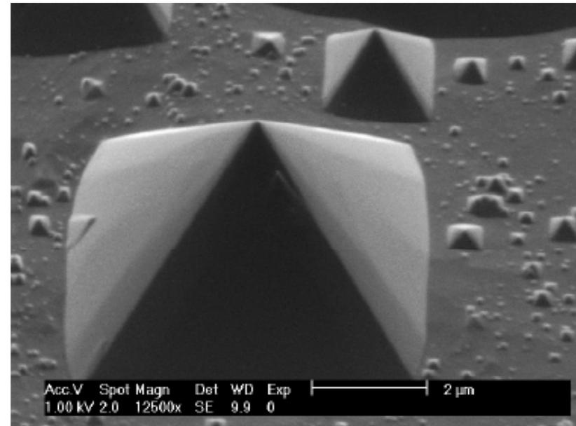
Examples of hillocks after Si wet etching using TMAH solution
