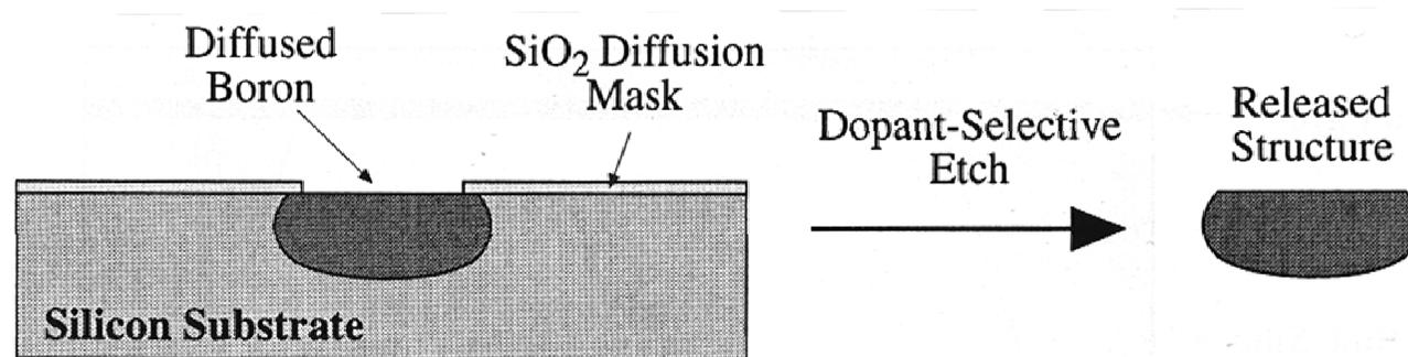
Illustration of the use of heavy boron doping with a dopant-selective etch to form free structures
