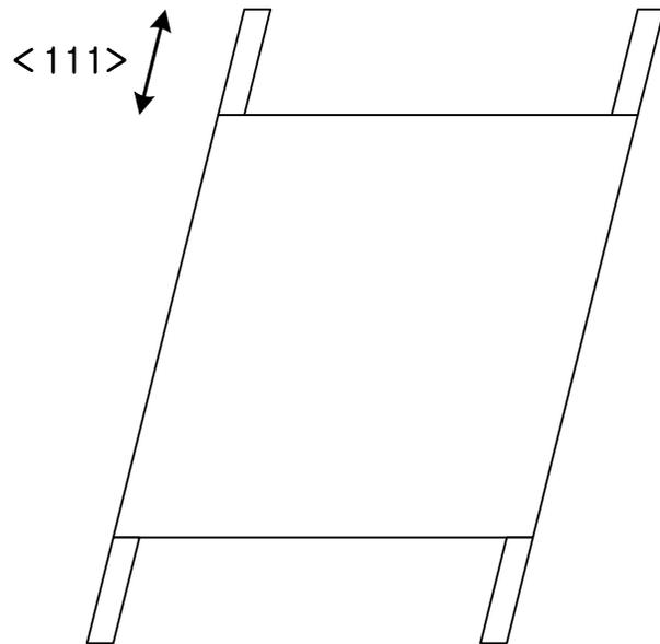
$\langle 111 \rangle$  direction compensation beams oblique to the wafer flat
