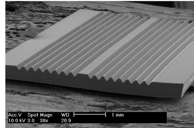
Example of anisotropic wet etching:
