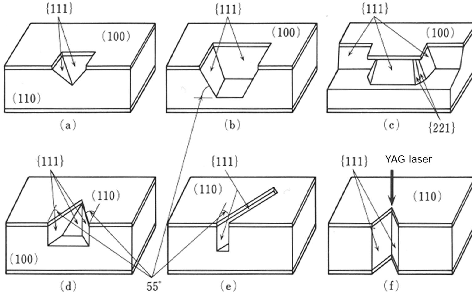
Silicon anisotropic wet etching of (100) and (110) silicon
