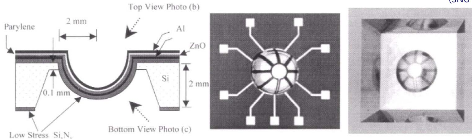
Example of isotropic wet etching: dome shaped diaphragm microphone
