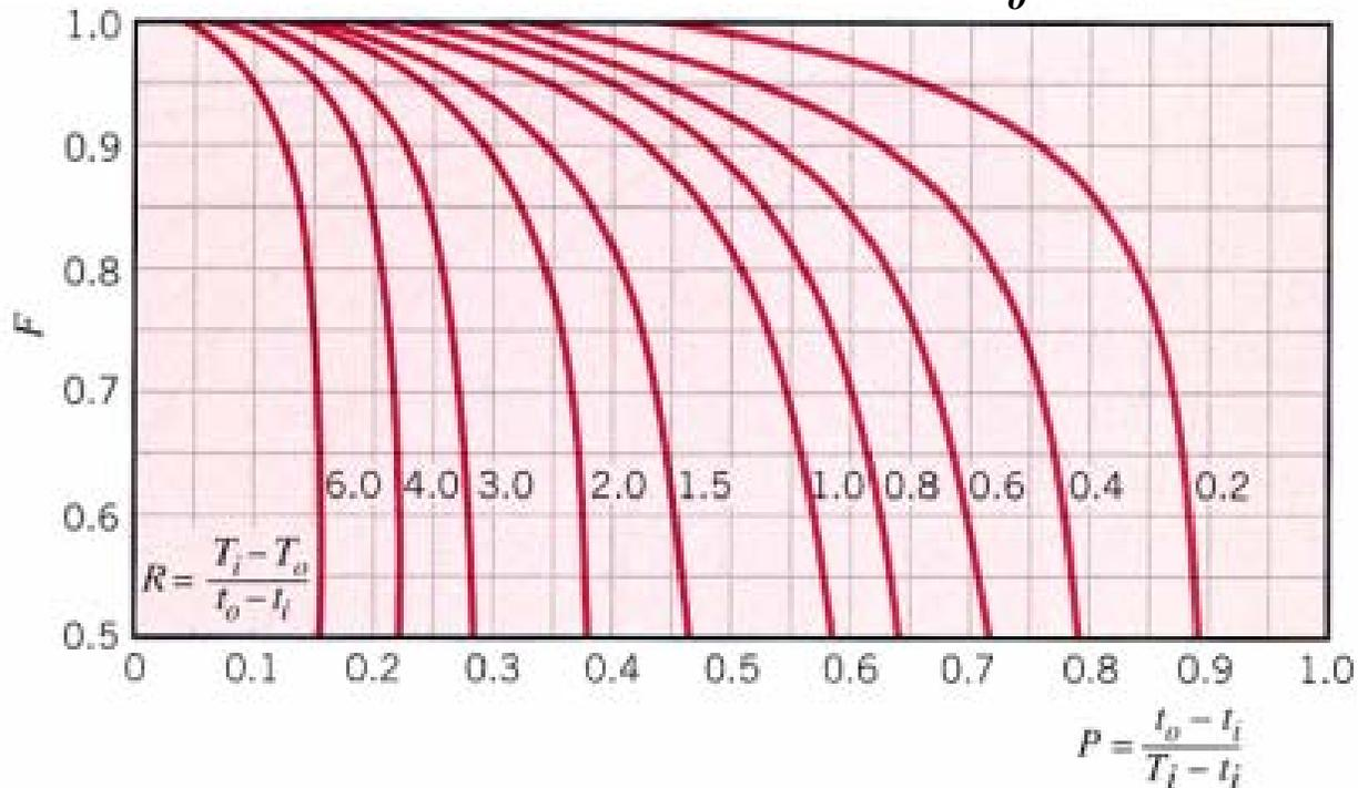
**FIGURE 11.10** Correction factor for a shell-and-tube heat exchanger with one shell and any multiple of two tube passes (two, four, etc. tube passes).
