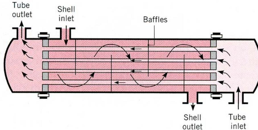
The main purpose of the baffles is to minimize channeling by which some of the fluid flows preferentially in certain paths that have little contact with the heat transfer surface. Each baffle may extend to half of the shell cross section; they are spaced at distances as close as one-fifth of the shell diameter.
