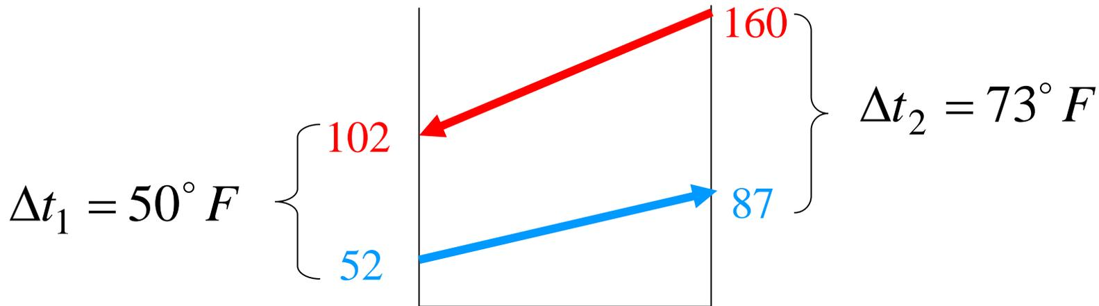
$$\therefore A_0 = \frac{q}{Y \cdot U_0} \frac{\ln(\Delta t_2 / \Delta t_1)}{\Delta t_2 - \Delta t_1} = \frac{(100,000)}{(0.89)(5.5)} \frac{\ln 73/50}{73 - 50} = 336(ft^2)$$
