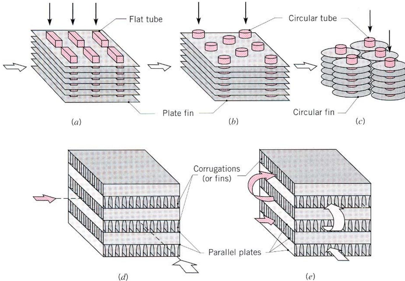
**FIGURE 11.5** Compact heat exchanger cores. (a) Fin-tube (flat tubes, continuous plate fins). (b) Fin-tube (circular tubes, continuous plate fins). (c) Fin-tube (circular tubes, circular fins). (d) Plate-fin (single pass). (e) Plate-fin (multipass).
