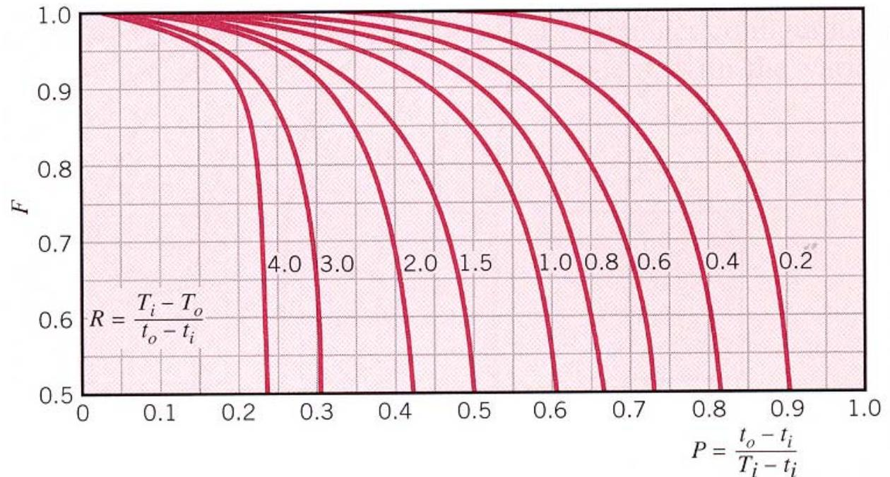
**FIGURE 11.13** Correction factor for a single-pass, cross-flow heat exchanger with one fluid mixed and the other unmixed.
