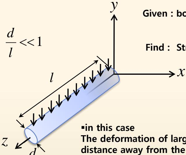
Given : body force  $Z = 0$ ,  $X = X(x, y)$ ,  $Y = Y(x, y)$
