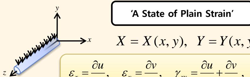
$$\varepsilon_x = \frac{\partial u}{\partial x}, \quad \varepsilon_y = \frac{\partial v}{\partial y}, \quad \gamma_{xy} = \frac{\partial u}{\partial y} + \frac{\partial v}{\partial x}, \quad \varepsilon_z = \gamma_{xz} = \gamma_{yz} = 0$$
