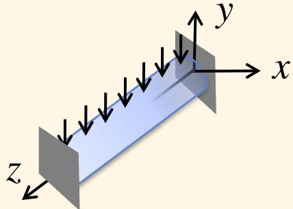
If the ends of the cylinder are prevented from moving in the \$z\$ coordinates, we can assume \$w=0\$ at every cross section of the cylinder
