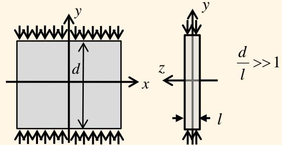
A thin plate under the lateral load uniformly distributed over its thickness
