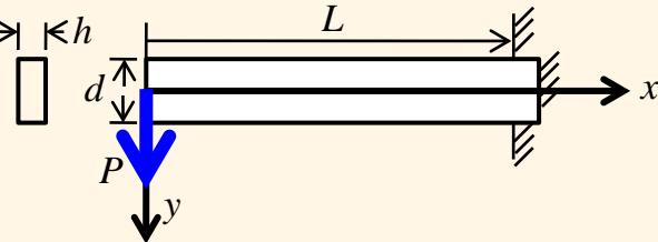
A cantilever beam of narrow rectangular cross section under an end load  $P$ . With its width  $h$  small compared with the depth  $d$ , the loaded beam may be regarded with as an example in plane stress
