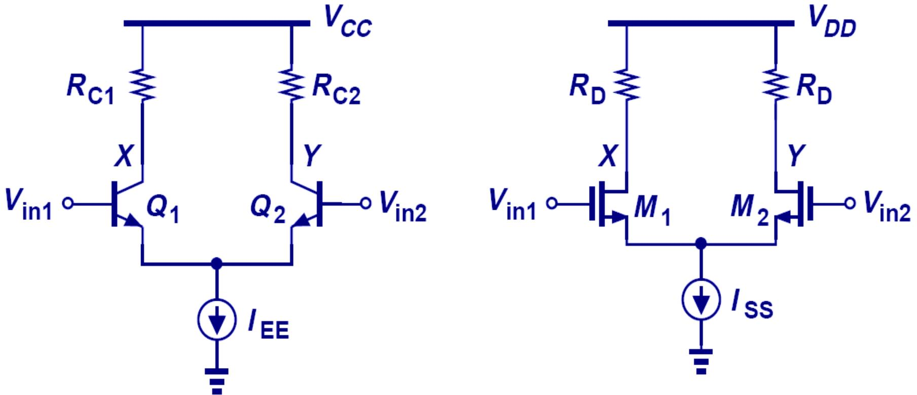
➤ With the addition of a tail current, the circuits above operate as an elegant, yet robust differential pair.
