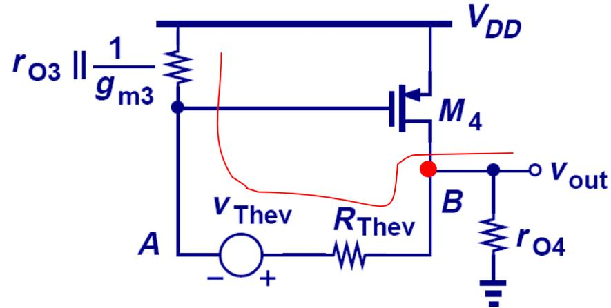
$$\Rightarrow \left( g_{m4} \frac{\frac{1}{g_{m3}} \parallel r_{O3}}{\frac{1}{g_{m3}} \parallel r_{O3} + R_{Thev}} + \frac{1}{\frac{1}{g_{m3}} \parallel r_{O3} + R_{Thev}} \right) (v_{out} + v_{Thev}) + \frac{v_{out}}{r_{O4}} = 0$$
