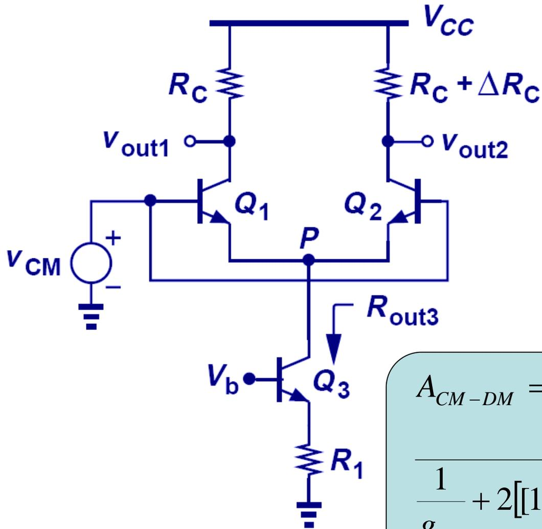
$$\therefore \left| \frac{\Delta V_{out}}{\Delta V_{CM}} \right| = \frac{\Delta R_C}{1/g_{m1} + 2R_{out3}}$$
