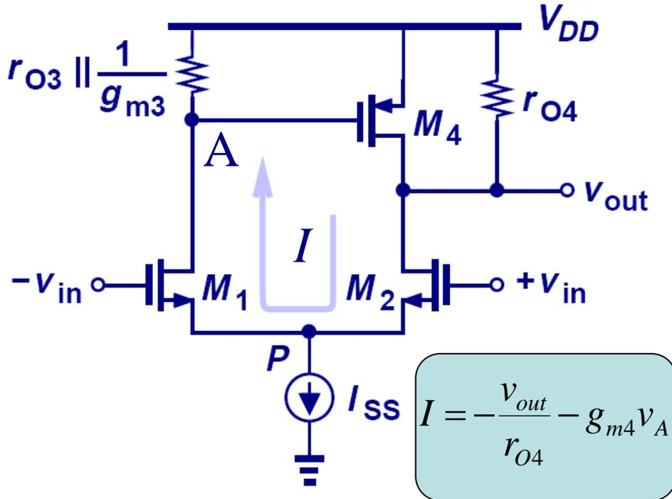
$$v_A = -\left(\frac{v_{out}}{r_{O4}} + g_{m4}v_A\right)\left(\frac{1}{g_{m3}} \parallel r_{O3}\right)$$
