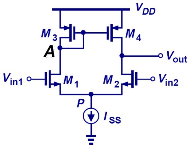
$$i_X = -i_Y \quad \& \quad v_A = -i_X \left( g_{mP}^{-1} \parallel r_{OP} \right)$$
