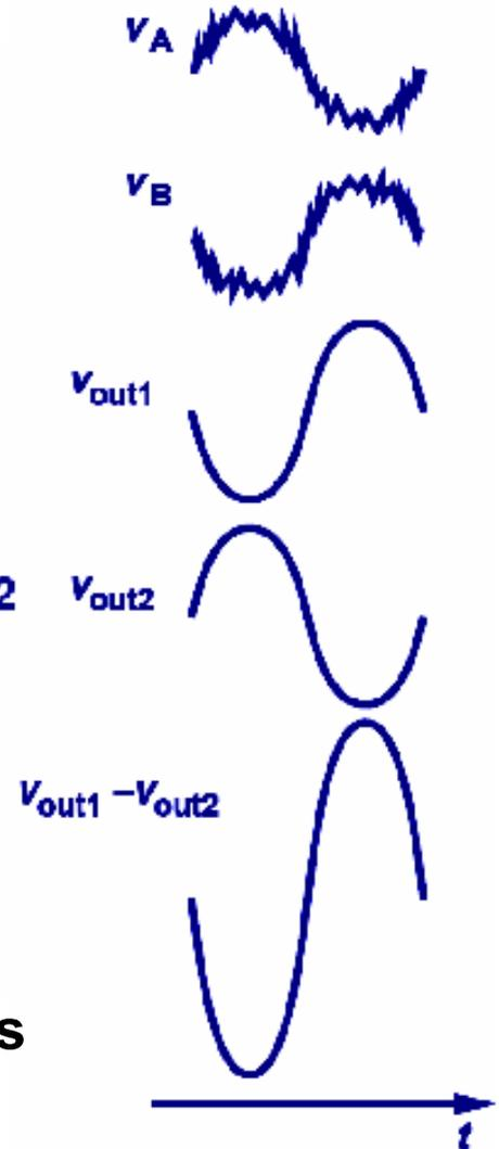
Change of CM input voltage can change  $V_P$ , but  $I_{EE}$  is constant due to infinite internal impedance
