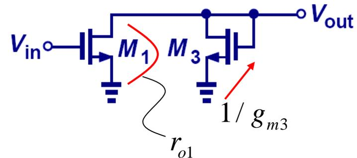
$$\frac{1}{g_{m3}} \parallel r_{o1} \approx \frac{1}{g_{m3}} \text{ due to } r_{o1} \gg \frac{1}{g_{m3}}$$
