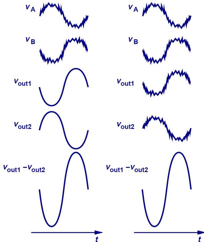
➤ As it can be seen, the differential output voltages for both cases are the same. So for small input CM noise, the differential pair is not affected.
