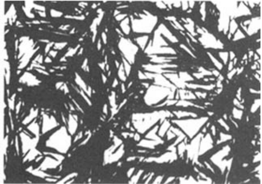
"Needle like" Structure of martensite
