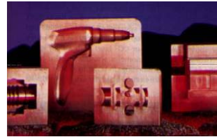
Core and cavity sets produced by RapidTool™
