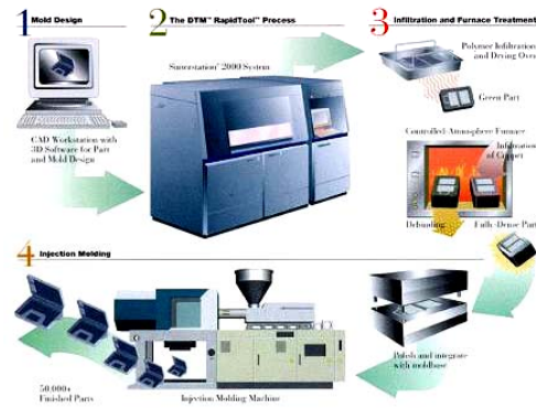
DTM's RapidTool™ process for rapid mold making
