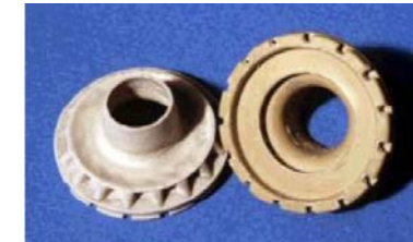
Silicon nitride parts fabricated using mold SDM process
