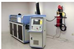
Helysis 2030E LOM machine Part envelope size 32"x22"x20"
