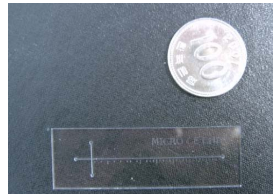
Microchip by direct machining
