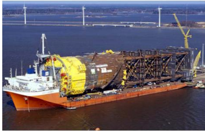
Dry-transport of Spar Hull
