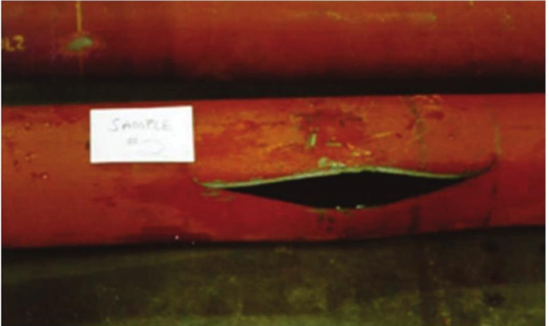
Figure A.1—Ductile Burst Sample
