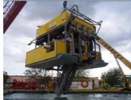
(b) Water Jet Trencher
