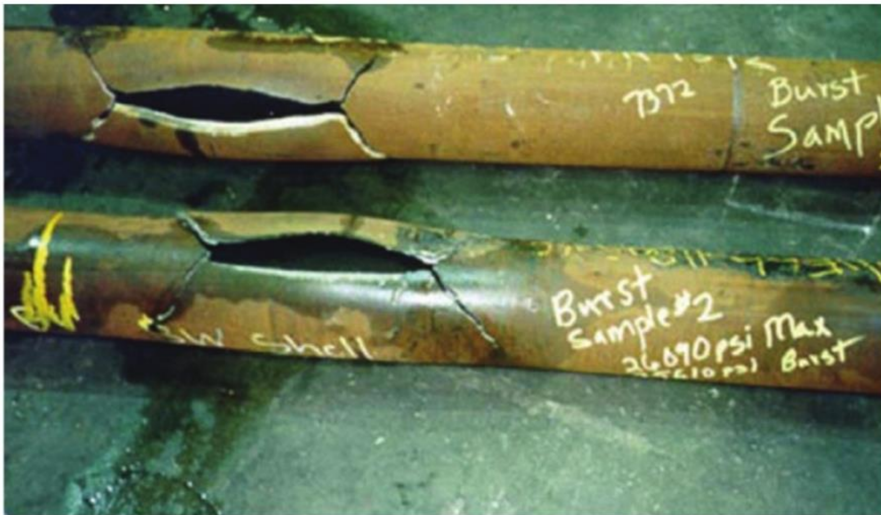
Figure A.2—Brittle Burst Sample
