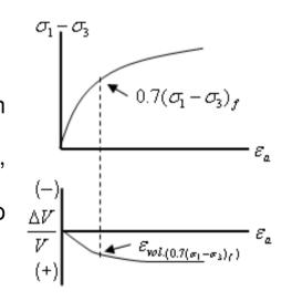
2) If the slope of the volume change curve = 0 before  $0.7(\sigma_1-\sigma_3)_f$  stress level is reached, then use the  $(\sigma_1-\sigma_3)$  and  $\varepsilon_{vol.}$  at that point to compute K<sub>B</sub>.
