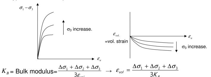
$K_B$  is a function of  $\sigma_3$  and it is independent of stress level  $(\sigma_1 - \sigma_3)$ .  $K_B$  is not changed by increase of loading.
