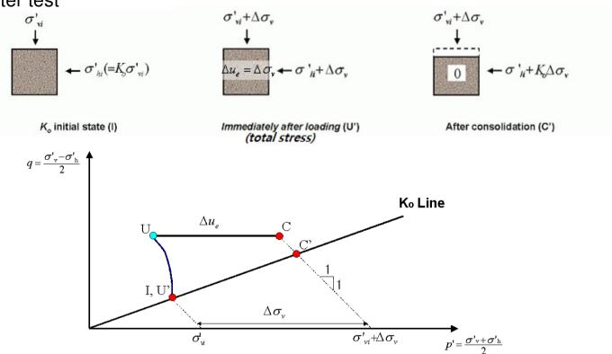
U'C': Consolidation path of oedometer test.
