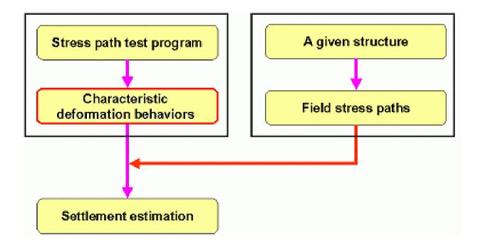
→ Characteristic behaviors of deformation which can cover all probable field stress paths are evaluated in advance by an economically-designed experimental program.
