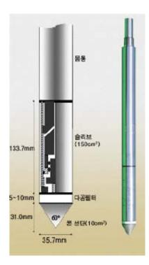
The CPT is carried out by pushing a  $60^{\circ}$  cone with a face area of  $10 \text{ cm}^2$  into the ground at a constant speed  $(2\pm0.5\text{cm/s})$ , whilst measuring the force to do so. The shear force on a  $150 \text{ cm}^2$  'friction sleeve' and pore pressure are then also measured.
