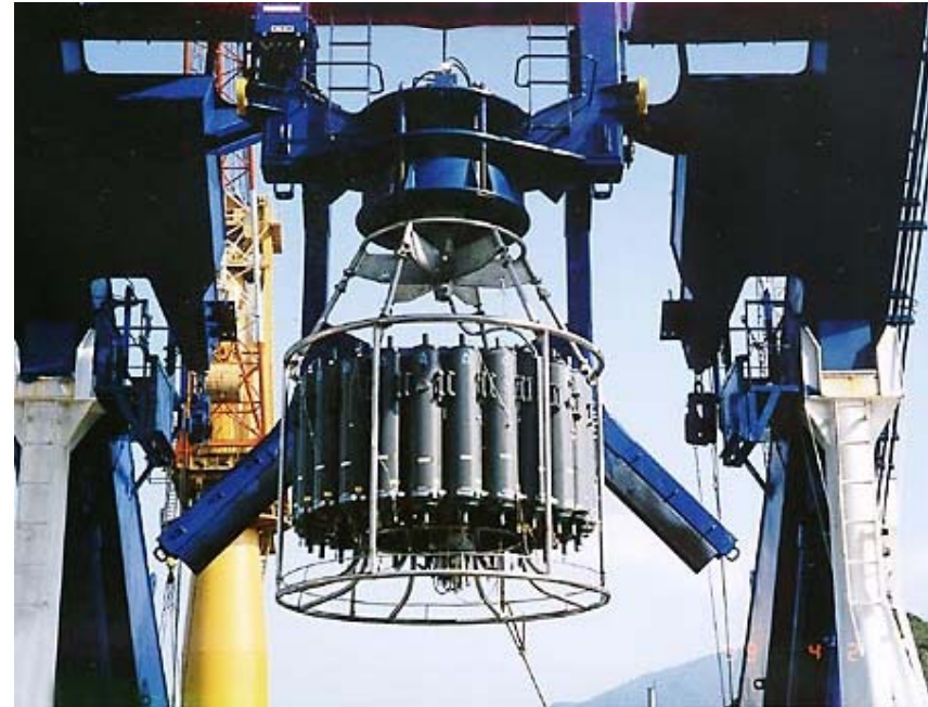
Rosette-Sampler with CTD Sensors
