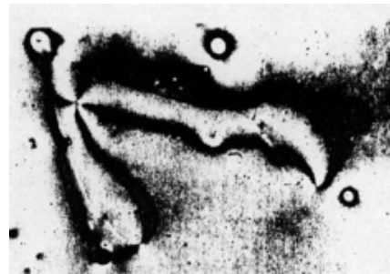
Figure 12 A typical nematic texture between crossed polarizers. [Q: Identify the two disclinations where two brushes meet and try to explain their origin (draw the director lines)].
