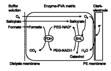
[Schematic representation of the PEG-NAD= regeneration system. (FDH, formate dehydrotenase; SHL, salicylate hydroxylase)]
