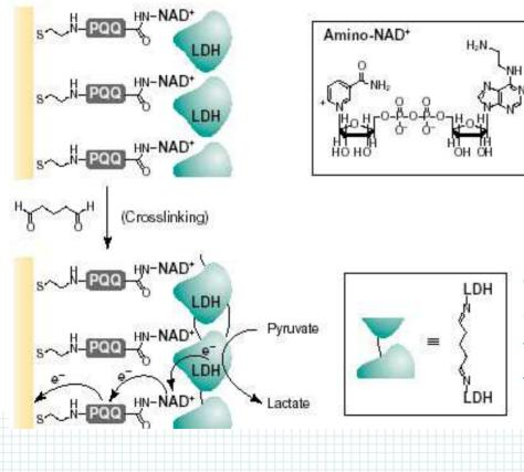
\* The enzyme-electrode stimulates the biocatalytic oxidation of lactate and act as an amperometric biosensor for lactate.
