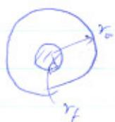
$$V_f = \frac{\pi r_f^2 L}{\pi r_a^2 L} = \frac{r_f^2}{r_a^2}$$
