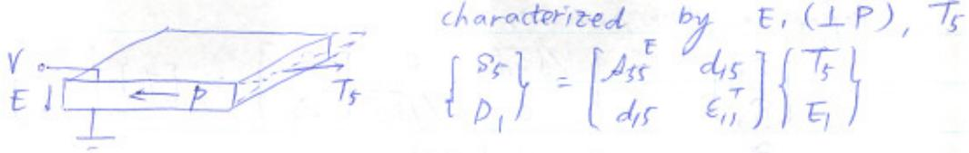
$$\begin{Bmatrix} S_5 \\ D_1 \end{Bmatrix} = \begin{bmatrix} d_{55}^E & d_{55}^T \\ d_{55}^T & \epsilon_{11}^T \end{bmatrix} \begin{Bmatrix} T_5 \\ E_1 \end{Bmatrix}$$
