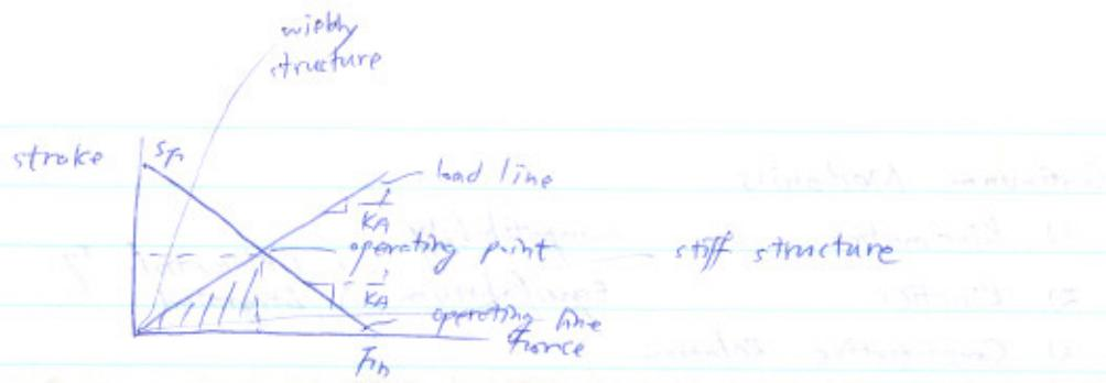
$$\text{max. work developed} : \frac{1}{2} \cdot \frac{1}{2} \epsilon_a^{\text{free}} \sigma_a^{\text{blocked}}$$
