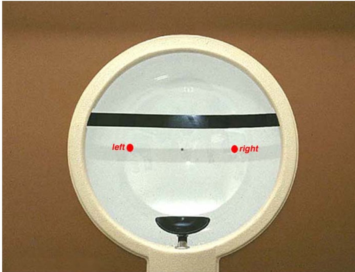
Fig. 46. Ganzfeld used for stimulating EOG recordings.
